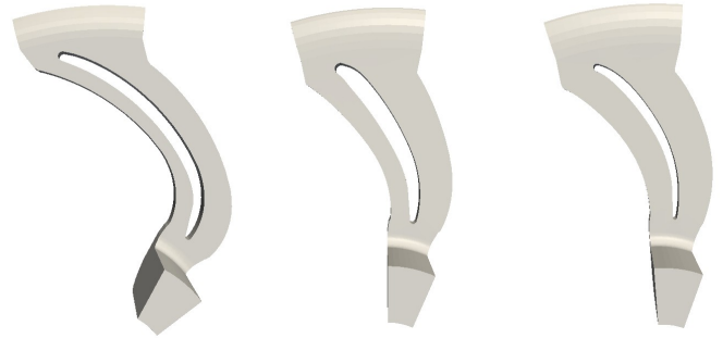
Figure 14 Left and middle: two random examples of geometries of generated during the preparation of random base, right: one of best examples being optimised for the run including U-turn optimisation.
