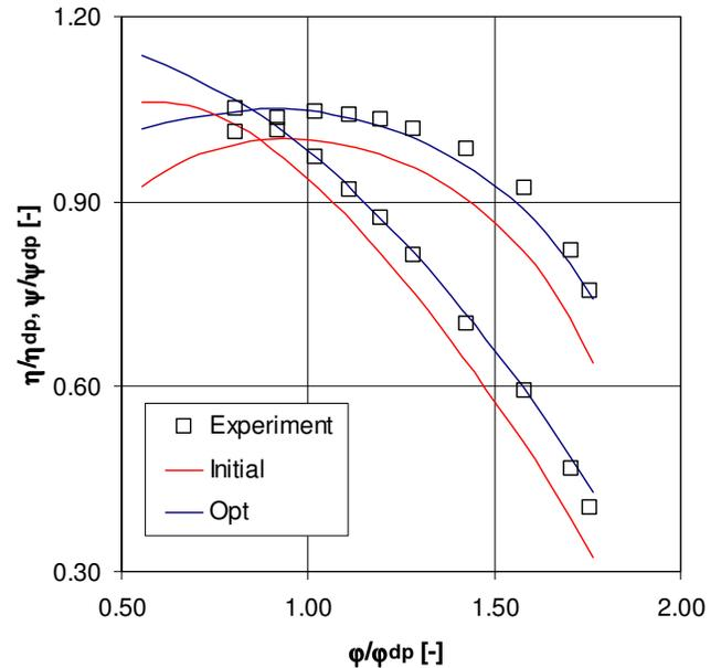
**Figure 7 Optimization results for polytropic efficiency and head**
