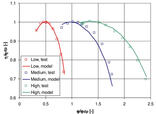
**Figure 1 Comparison between predicted and tested efficiency**
