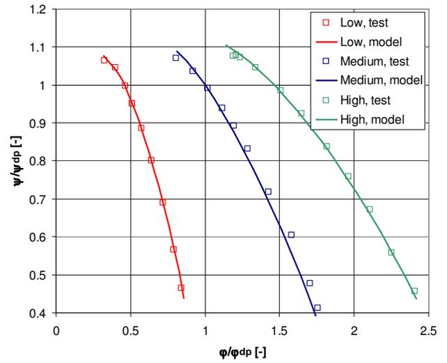
Figure 2 Comparison between predicted and tested head
