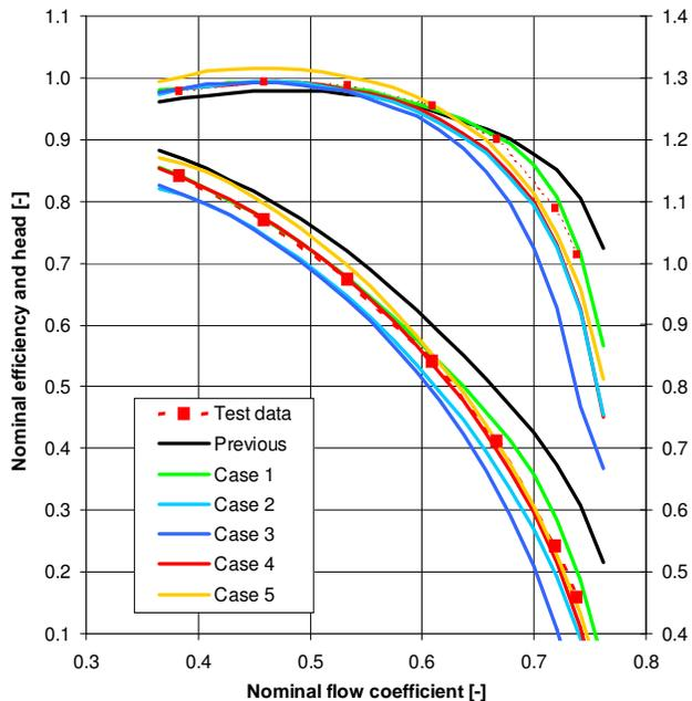
**Figure 11 Result of tuning options on one master and one speed line**
