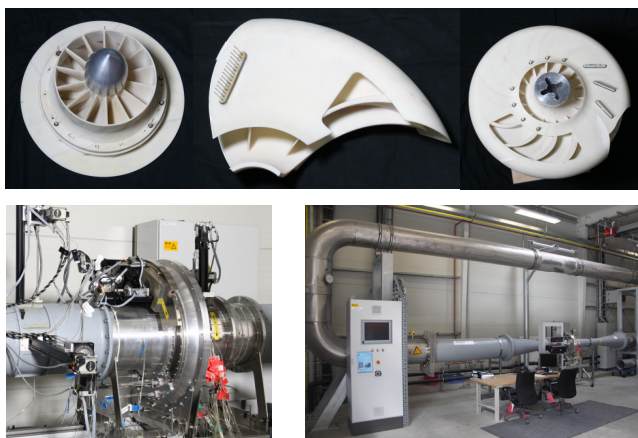
Figure 4: Top: Photographs of the cascade segments. From left to right: preswirler section, return channel segment and assembled return channel section. Bottom: Photographs of test section (left) and overall test facility (right).
