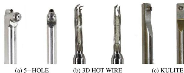
**FIGURE 3: PROBES USED FOR THE TRAVERSE PLANE INVESTIGATIONS**
