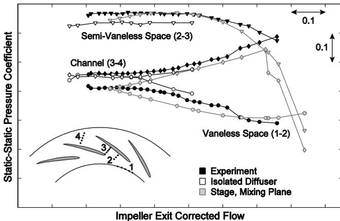
Figure 5: Subcomponent characteristics for 100% design corrected speed.
