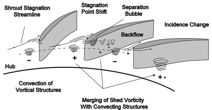
**Figure 17: Suggested mechanism for short-wavelength stall inception in vaned diffusers.**
