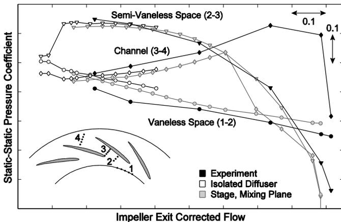
Figure 6: Subcomponent characteristics for 78% design corrected speed.
