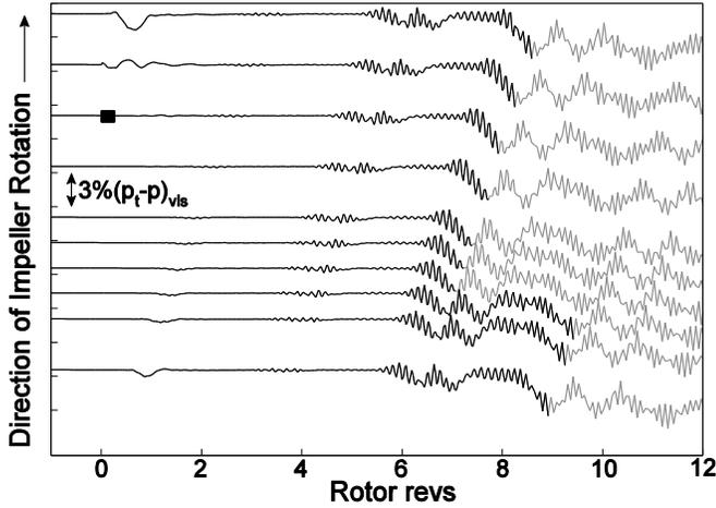
**Figure 11: Computed static pressure traces in the vaneless space at 100% design corrected speed for the operating point at 90%  $\dot{m}_{c,PDPR}$ . The small black box represents duration and spatial extent of the initial forcing function.**
