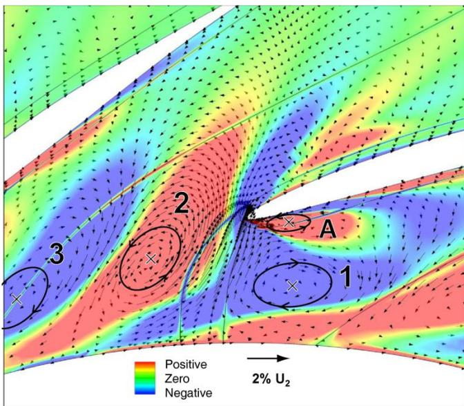
**Figure 9: Time snapshot of counter-rotating vortical structures 1, 2 and 3 convecting in vaneless space at 90% span. Vorticity shed from leading edge (A) merges with passing vortical structure 2 at a later time.**
