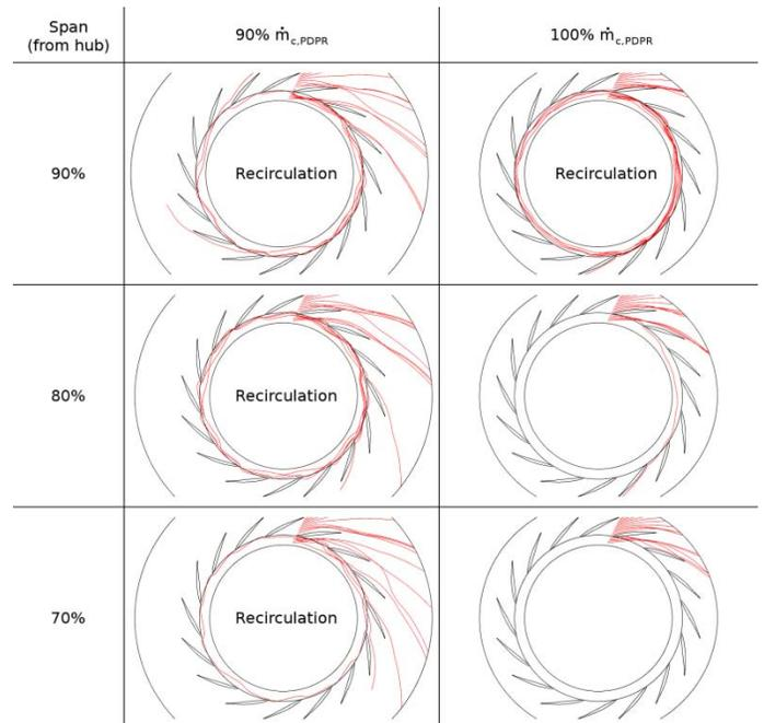
**Figure 10: Flow near shroud recirculates in the vaneless space over a larger spanwise extent as diffuser inlet corrected flow is reduced; combined with separation from the vane leading edge, conditions on left allow short wavelength stall inception.**
