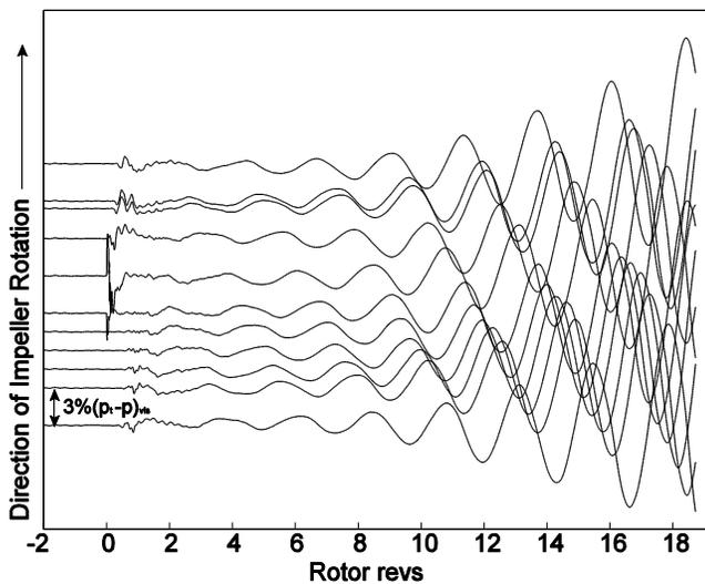
**Figure 16: Computed static pressure traces in the vaneless space using full wheel body force simulation at 75% design speed, adapted from [18]. Backward traveling modal waves are observed prior to stall.**
