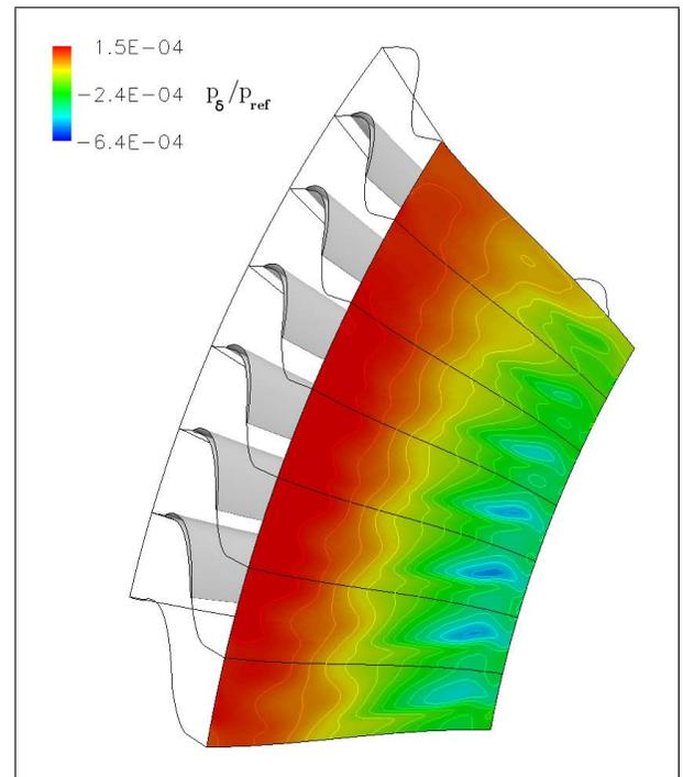
FIGURE 11. Acoustic pressure perturbation at turbine exit (+1V1-1B1 interaction)
