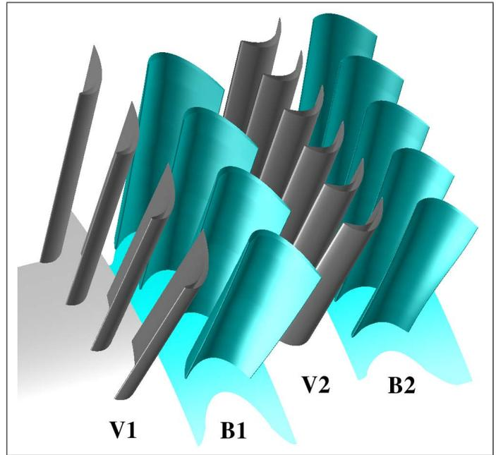
FIGURE 5. Cold-flow rig: geometry of the blades
