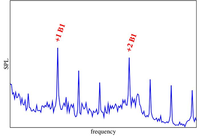
FIGURE 2. Measured noise spectrum and tone identification
