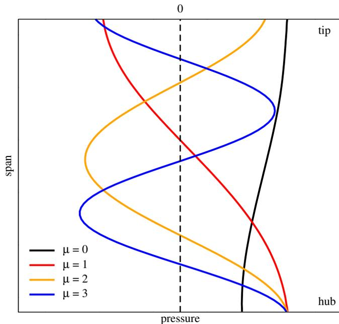
**FIGURE 3. Radial mode shapes (in terms of pressure) at B2 exit for +2B1-1V2 mode**
