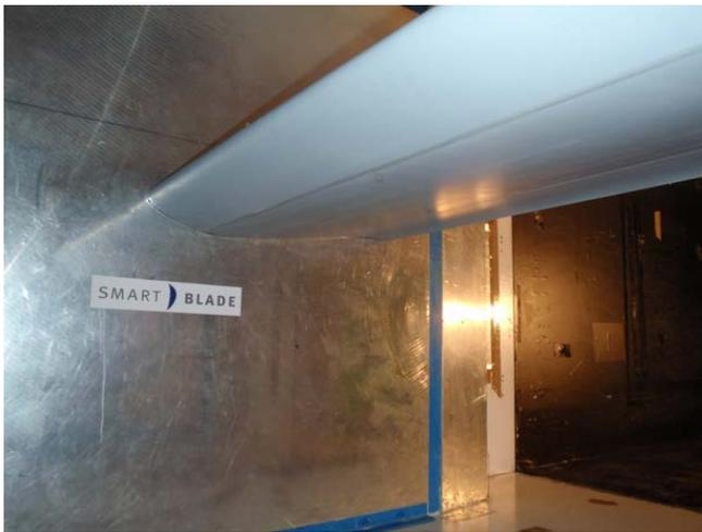
**FIGURE 13.** THE  $NACA63_3618$  TEST WING WITH THE FLEXIBLE LEADING EDGE FLAP IN THE WIND TUNNEL.
