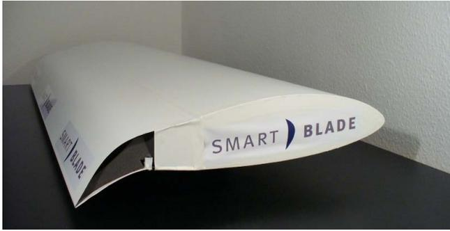
**FIGURE 4.** THE DU96W180 TEST WING WITH THE FLEXIBLE FLAP AT FULL DEFLECTION.
