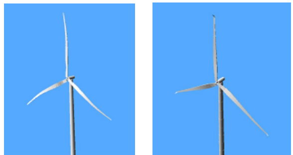
Figure 1 (a) highly swept blades, (b) blades with winglets
