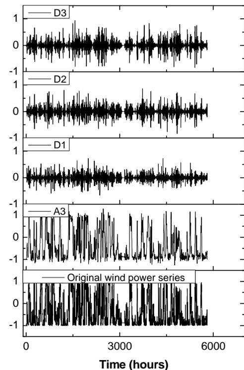
**Figure 11.** Six Daubechies wavelet decomposition (level 3) of the original wind power series (normalized values)
