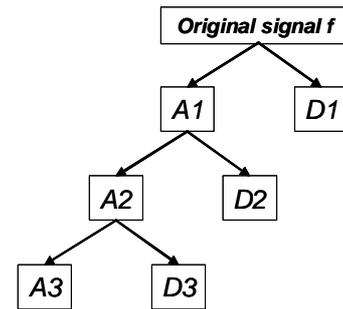
**Figure 9.** Multilevel decomposition process of the original hourly wind power time series ( $f$ ): A and D stand for approximation and detail, respectively ( $f = A3 + D1 + D2 + D3$ )
