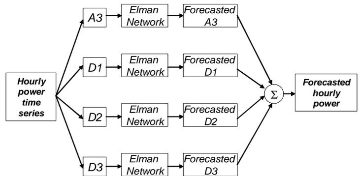
**Figure 10.** Architecture of the forecast approach based on the wavelet decomposition technique
