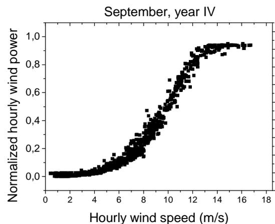
Figure 3. Normalized hourly wind power vs hourly wind speed in the month of September, year IV
