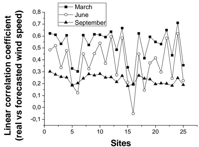
**Figure 5.** Linear correlation coefficient between the real hourly average wind speed and the forecasted one, year V
