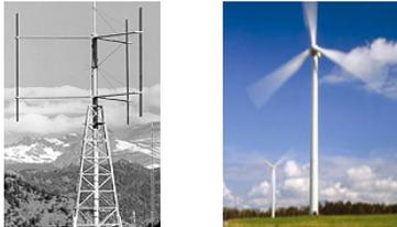
Figure 6. Wind turbine: a) VAWT and b) HAWT
