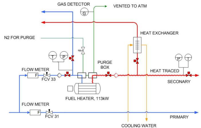
Figure 3: Process and instrumentation diagram of fuel heating & supply system.
