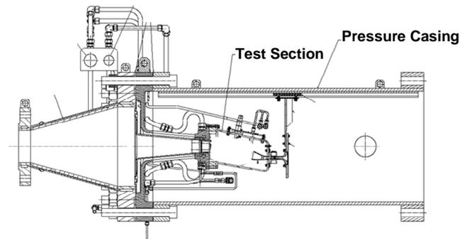
(a) Combustor Test Section
