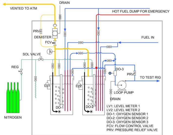
Figure 1: Process & Instrumentation Diagram of the fuel sparging system
