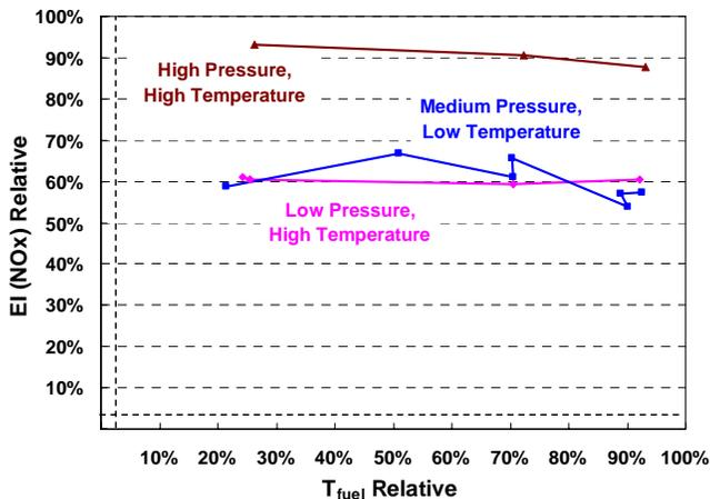
Figure 8: Fuel temperature effect on relative EI NOx
