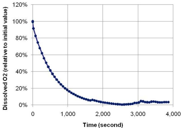
Figure 2: Change of dissolved oxygen level by the sparging process
