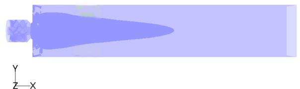
Figure 5. VBB of the single-element LDI combustor (side view)
