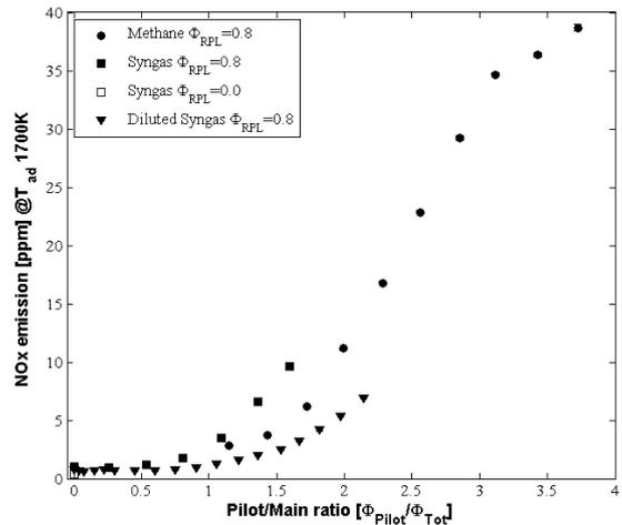
Figure 10: NO<sub>x</sub> with fuel partitioning, Pilot divided by total equivalence ratio.
