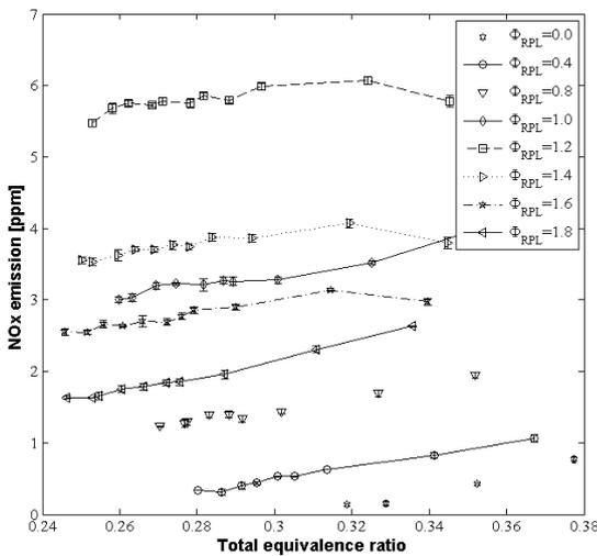
Figure 6: Syngas, NO<sub>x</sub> emission with total equivalence ratio for relevant RPL equivalence ratios.
