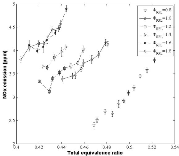
Figure 5: Methane, NO<sub>x</sub> emission with total equivalence ratio for relevant RPL equivalence ratios.
