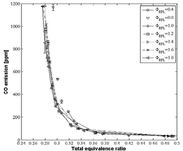
**Figure 4: Dilute syngas, CO emission with total equivalence ratio for relevant RPL equivalence ratios.**
