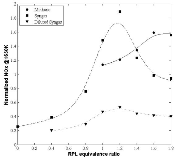
Figure 8: NO<sub>x</sub> emission for relevant RPL equivalence ratios, total flame temperature 1650 K.
