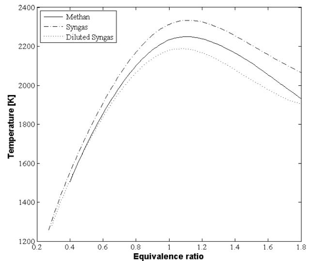
Figure 3: Temperature from PSR, 1.5 ms residence time
