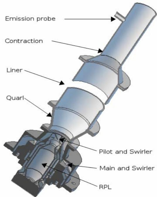
**Figure 1: Burner Assembly**
