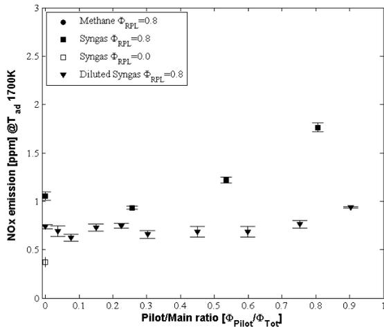
Figure 9: NO<sub>x</sub> emission, fuel partition weighted to Main burner sector.
