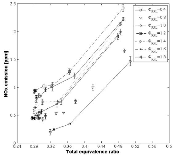
Figure 7: Dilute syngas, NO<sub>x</sub> emission with total equivalence ratio for relevant RPL equivalence ratios.
