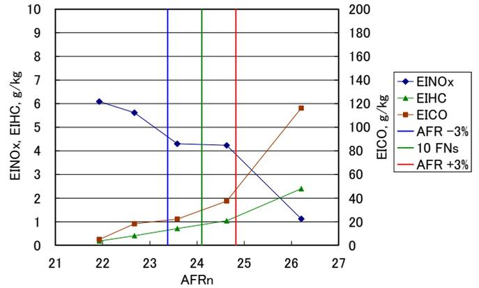
Figure 7. DEPENDENCE OF EMISSION INDICES ON THE AFR BASED ON THE AIR FLOW RATE OF THE FUEL NOZZLE AT PRESSURE AND TEMPERATURE OF 85% MTO CONDITION.
