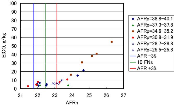
Figure 10. DEPENDENCE OF CO EMISSION INDICES ON THE AFR BASED ON THE AIR FLOW RATE OF THE FUEL NOZZLE AT PRESSURE AND TEMPERATURE OF 100% MTO CONDITION.
