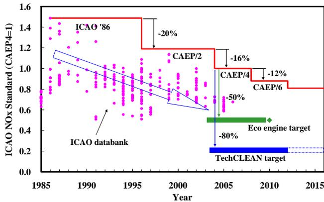
Figure 1. ICAO NO<sub>x</sub> STANDARD AND THE TARGET OF TECHCLEAN PROJECT.
