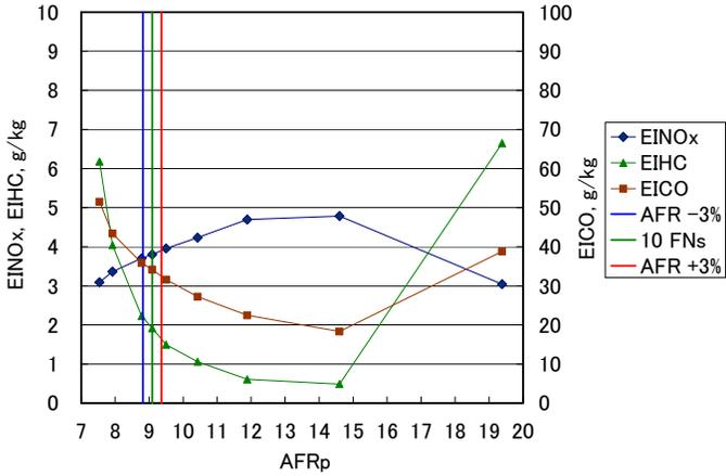
Figure 5. DEPENDENCE OF EMISSION INDICES ON AFR BASED ON THE AIR FLOW RATE OF THE PILOT AT PRESSURE AND AIR TEMPERATURE OF 7% MTO CONDITION.
