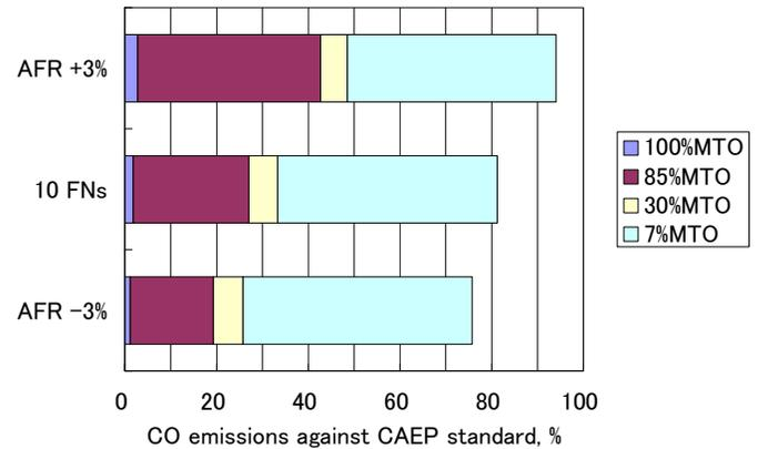
Figure 14. CO EMISSIONS AGAINST THE CAEP STANDARD AT LTO CYCLE CONDITIONS IN THREE AFR SETTINGS OF THE FUEL NOZZLE.
