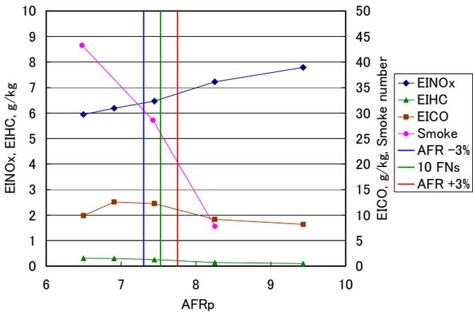
Figure 6. DEPENDENCE OF EMISSION INDICES ON THE AFR BASED ON THE AIR FLOW RATE OF THE PILOT AT PRESSURE AND TEMPERATURE OF 30% MTO CONDITION.
