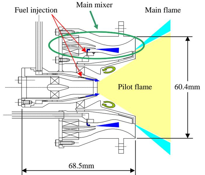
Figure 2. THE CROSS-SECTION OF THE FUEL NOZZLE MODEL E.
