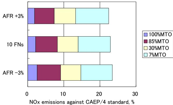
Figure 12. NOx EMISSIONS AGAINST THE CAEP/4 STANDARD AT LTO CYCLE CONDITIONS IN THREE AFR SETTINGS OF THE FUEL NOZZLE.
