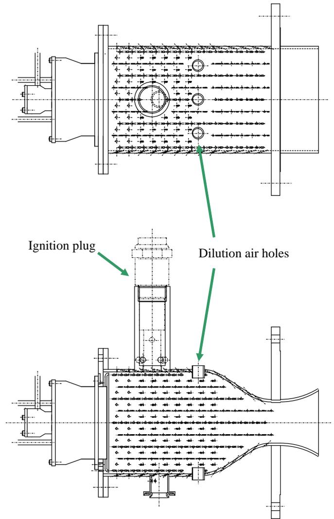
Figure 4. SCHEMATICS OF SINGLE-SECTOR COMBUSTOR
