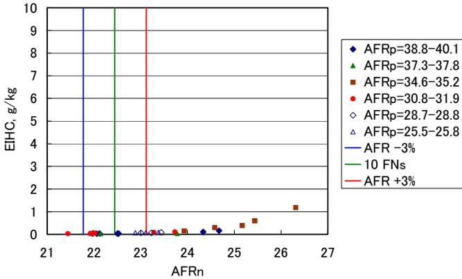
Figure 9. DEPENDENCE OF HC EMISSION INDICES ON THE AFR BASED ON THE AIR FLOW RATE OF THE FUEL NOZZLE AT PRESSURE AND TEMPERATURE OF 100% MTO CONDITION.
