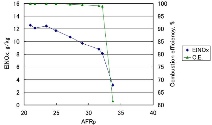
Figure 11. DEPENDENCE OF NO<sub>x</sub> EMISSION INDEX AND COMBUSTION EFFICIENCY ON THE AFR BASED ON AIR FLOW RATE OF PILOT MIXER AT PRESSURE AND TEMPERATURE OF 100% MTO CONDITION.
