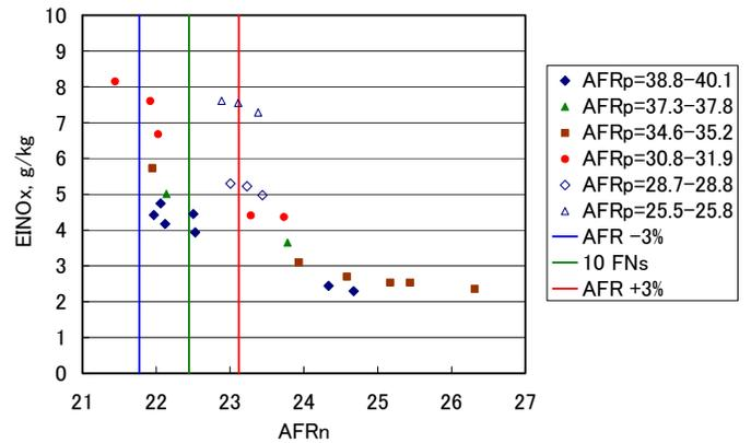
Figure 8. DEPENDENCE OF NO<sub>x</sub> EMISSION INDICES ON THE AFR BASED ON THE AIR FLOW RATE OF THE FUEL NOZZLE AT PRESSURE AND TEMPERATURE OF 100% MTO CONDITION.
