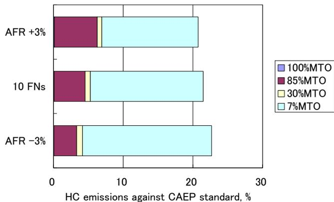
Figure 13. HC EMISSIONS AGAINST THE CAEP STANDARD AT LTO CYCLE CONDITIONS IN THREE AFR SETTINGS OF THE FUEL NOZZLE.
