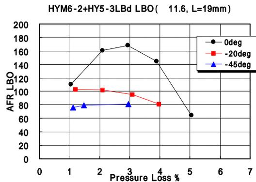
Figure 5 Single burner ignition / lean blow out result (Effect of inner swirler angle)
