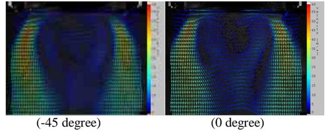
**Figure 8 Flow field by PIV measurement**
