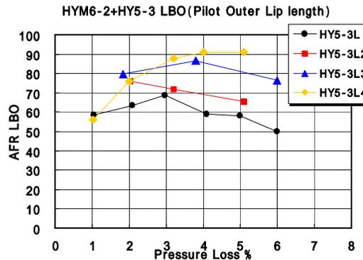
Figure 4 Single burner ignition / lean blow out result (Effect of pilot outer lip length)
