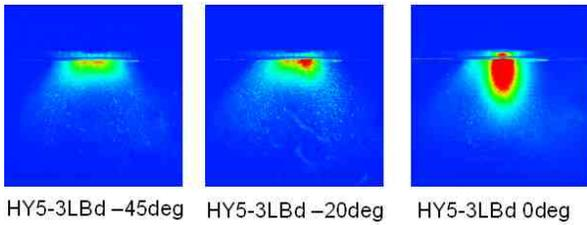
**Figure 7 Single burner pilot spray distribution (Effect of inner swirler angle)**
