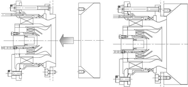
Figure 18 Fuel injector with the extended heat shield
