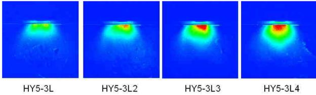
**Figure 6 Single burner pilot spray distribution (Effect of pilot outer lip length)**
