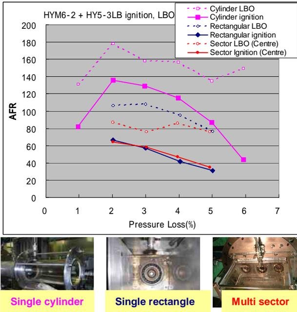
**Fig.15 Comparison of ignition and lean blow out characteristics in single cylindrical, single rectangle and multi sector unit.**
