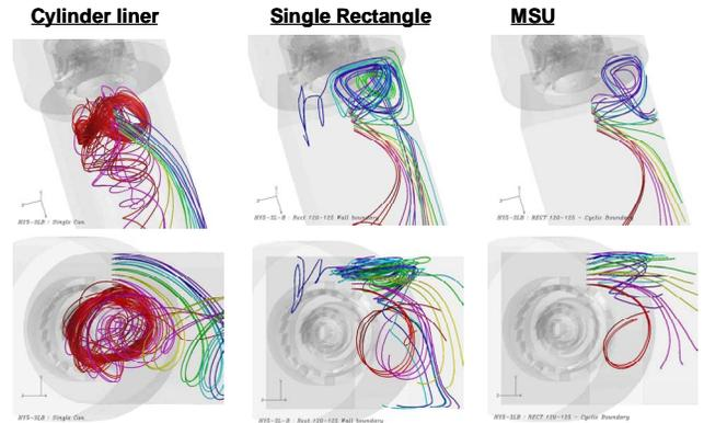
**Fig. 17 Flow field around igniter tip**
