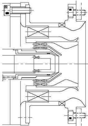
**Figure 1 Schematic view of lean staged fuel injector**
