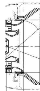
Figure 23 Extended heat shield with back side cooling system
