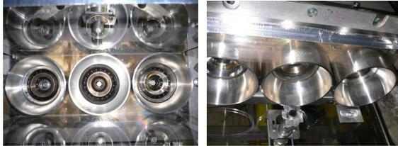
Figure 19 Fuel injector with the extended heat shield
