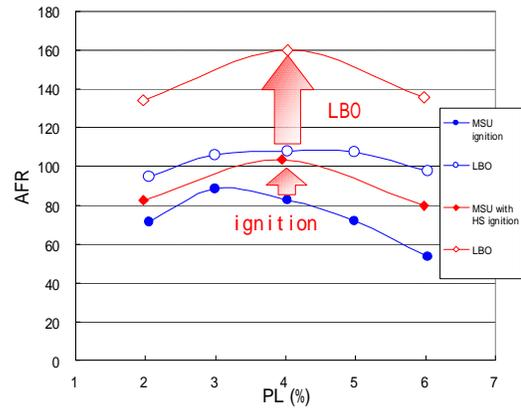
Fig.22 Improvement in performance with extended heat shield
