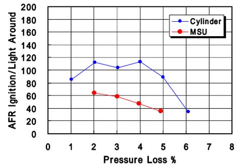
Fig. 14 Light around and lean blow out result in multi sector unit
