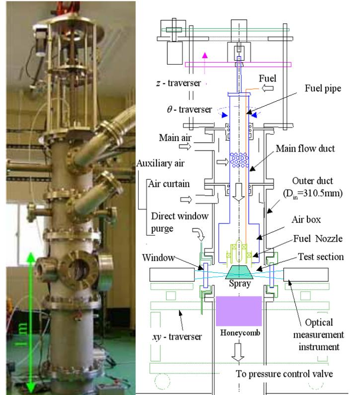
Figure 4: High pressure spray test facility
