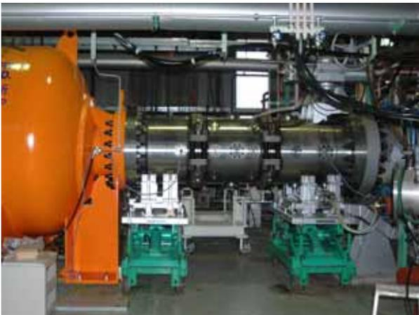
Figure 18: JAXA AP7 combustion test rig
