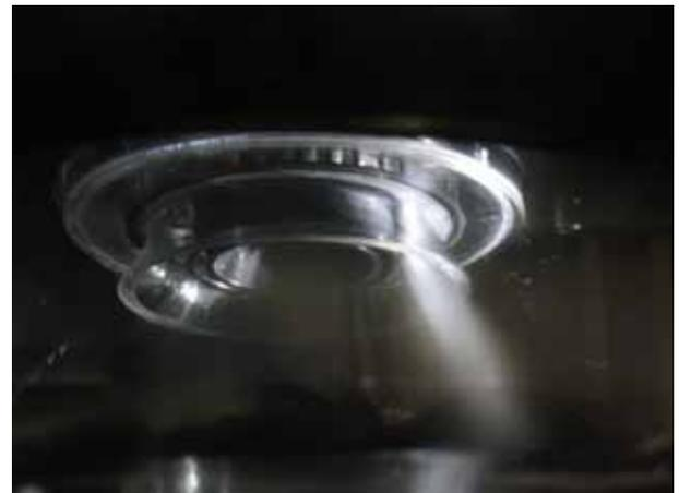
Figure 16: Spray of Type RS under IP condition
