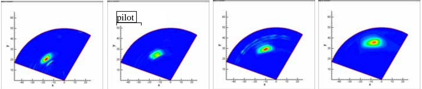
Figure 7: spray distribution of model AX at IP condition (Z=-14, -6, +2, +10mm)
