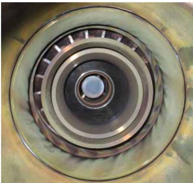
Figure 2: photograph of the concentric fuel nozzle (viewing from downstream after an HP combustion test)
