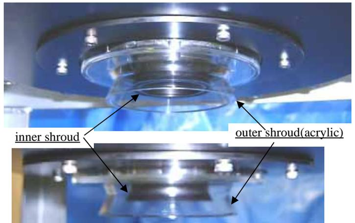
Figure 5: spray test model of the concentric fuel nozzle
