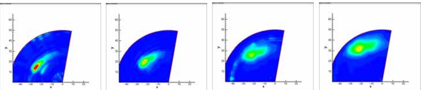
Figure 10: spray distribution of model RS at HP condition (Z=-14, -6, +2, +10mm)
