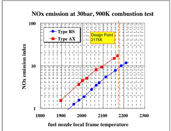
Figure 20 : NOx emission index obtained at 30bar, 900K Combustion test
