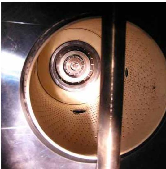
Figure 19 : the fuel nozzle, the liner and a gas sampling probe (viewing from downstream)
