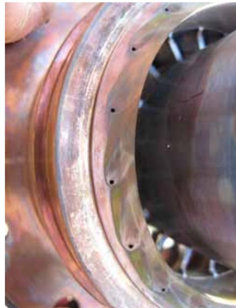
Figure 3: main fuel holes for RS direction (viewing from downstream after a HP combustion test)
