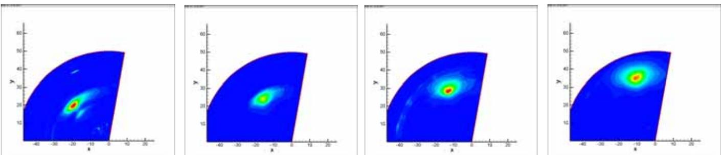
Figure 9: spray distribution of model RS at IP condition (Z=-14, -6, +2, +10mm)
