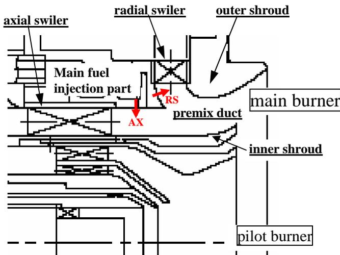
Figure 1: Cross sectional view of the concentric fuel nozzle
