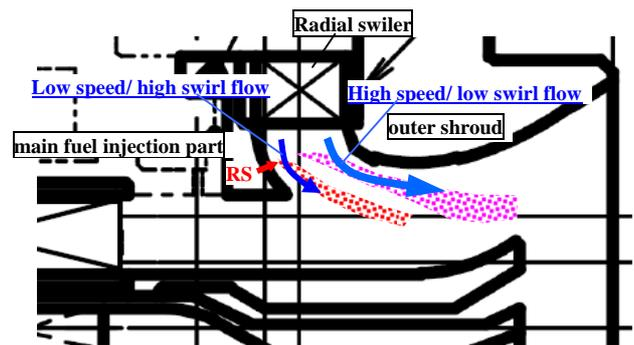
Figure 17: Flow field in the radial swirl flow
