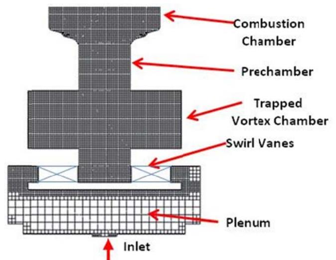
**Figure 5: CFD Model of the Rig Combustor with TVC feature**
