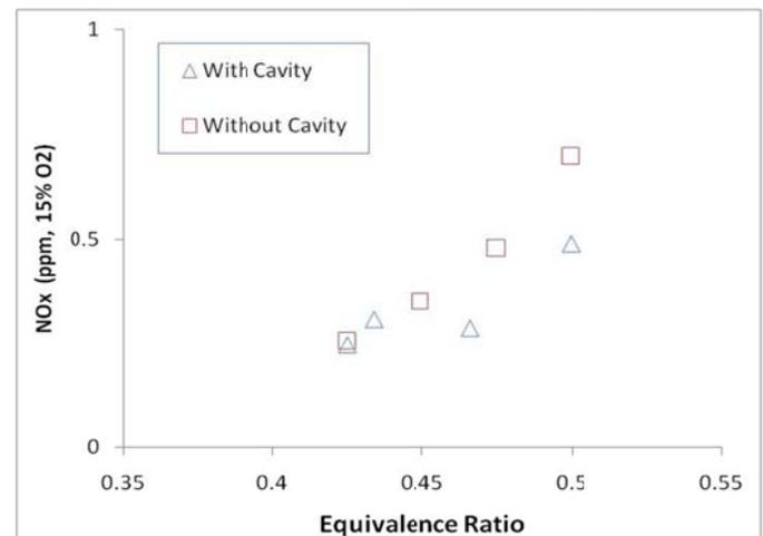
Figure 16: Actual (corrected for 15% O<sub>2</sub>) NO<sub>x</sub> as a Function of Equivalence Ratio for Combustor With and Without TVC for  $U_{mean}=30$  m/sec and Vane Thickness of 29.86 mm
