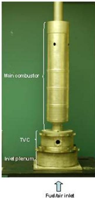
**Figure 4: Photograph of assembled combustion system**
