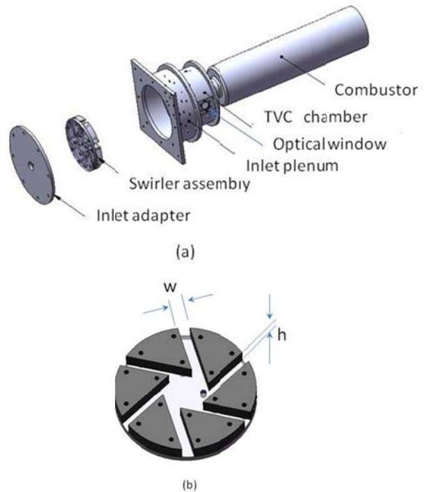
Figure 3: Modular Rig Design: (a) view of exploded combustor assembly and (b) radial swirler configuration
