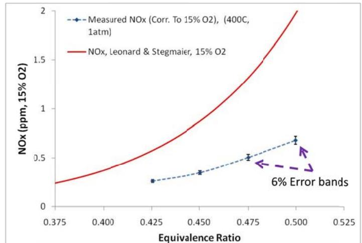
Figure 15: Corrected NO<sub>x</sub> (15% O<sub>2</sub>) as a function of Equivalence Ratio for Combustor without TVC
