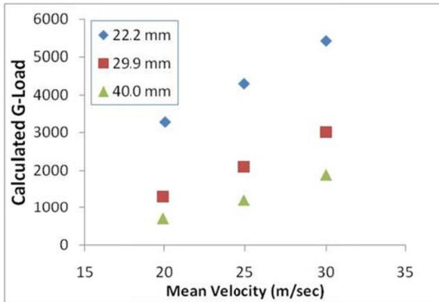
Figure 7: Effect of Vane Thickness of Swirler on ‘g-load’
