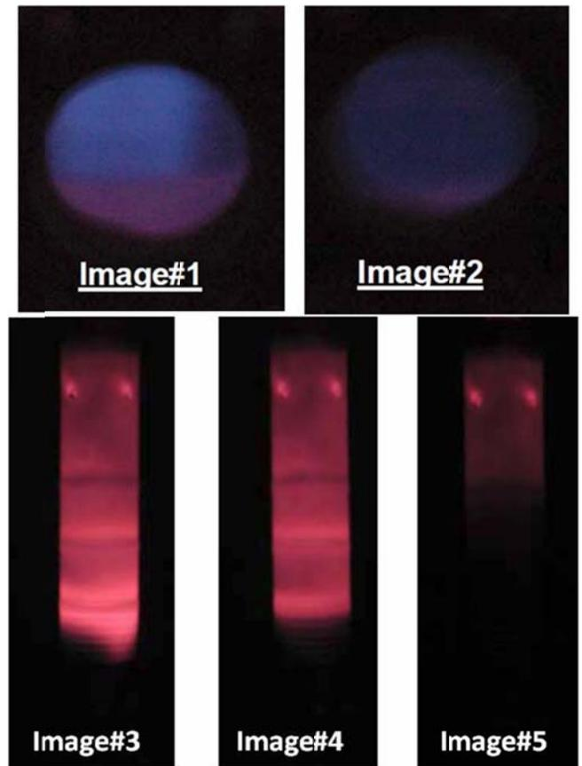
Figure 9: Images of Flame Characterization at 400C, g-load=1912, axial velocity = 30 m/s.
