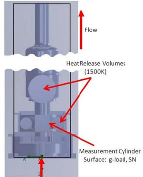
**Figure 6: CFD Model with virtual volumes to capture combustion heat release near lean blowout**
