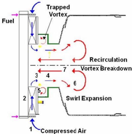
Figure 2: High G-load TVC Combustor Concept
