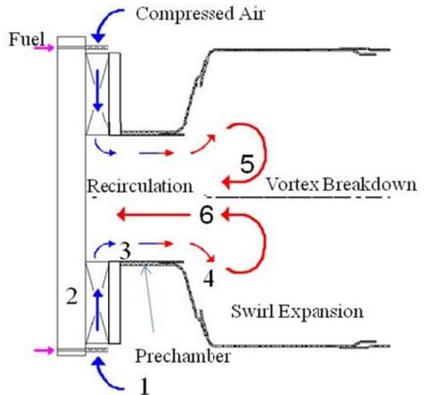
Figure 1: Baseline microturbine combustor
