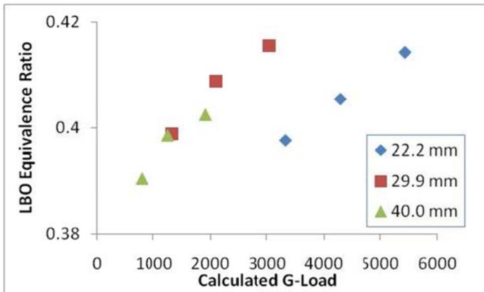
Figure 13: Lean Blow Out (LBO) Limit vs. G-load
