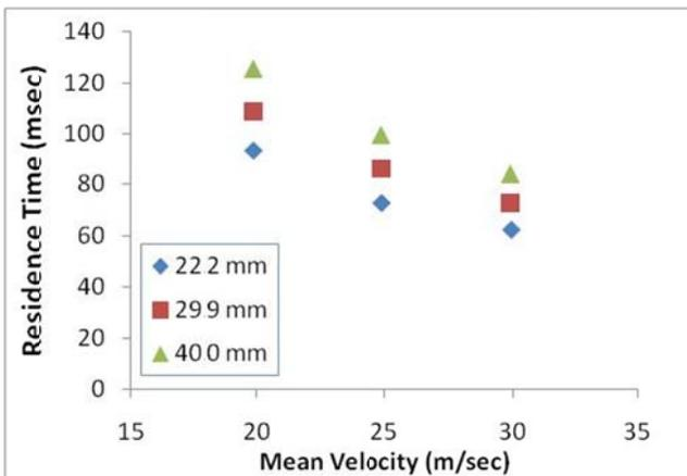
Figure 8: Effect of Vane Thickness of Swirler on Residence Time in Trapped Vortex Cavity
