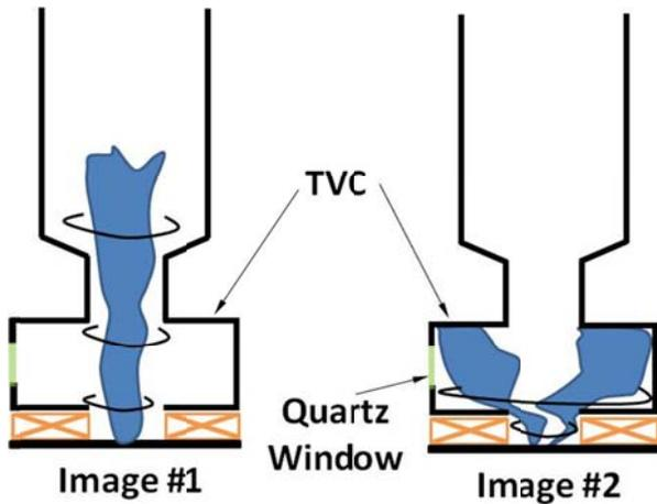
Figure 10: Schematic of observed flame shapes for Type I and Type II flame structures
