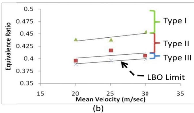
Figure 11: Maps of flame regime for various mean velocities for vanes with thickness of (a) 22.23 mm and (b) 40.01 mm
