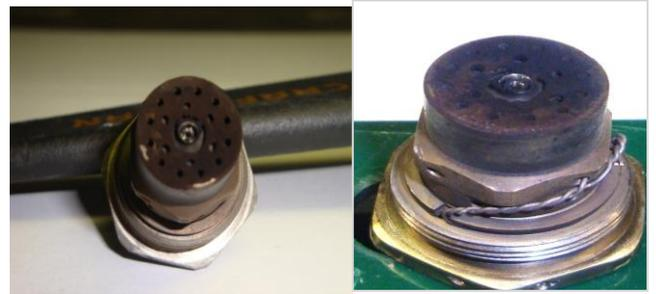
FIGURE 14. FUEL NOZZLE OF T63 ENGINE OPERATED ON: (a) HRJ BLEND FOR 150 HRS, (b) JP-8 FOR 175 HRS
