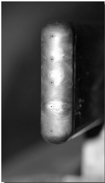
**Figure 2 – Leading edge of an old design gas analysis probes after tests (max. outlet temperature around 1950 K during 10h).**
