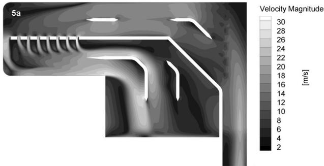
Figure 21 – Velocity magnitude of water inside the probe in case Sim2 on design #5.
