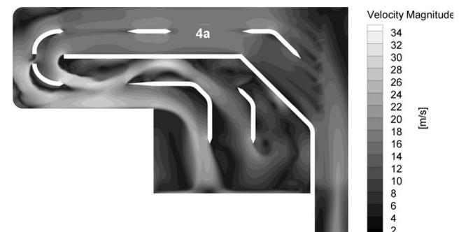
**Figure 20 – Velocity magnitude of water inside the probe in case Sim2 on design #4.**
