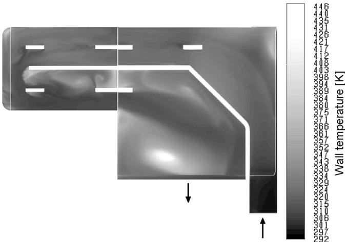
Figure 12 – Internal wall temperature of probe in case Sim2.
