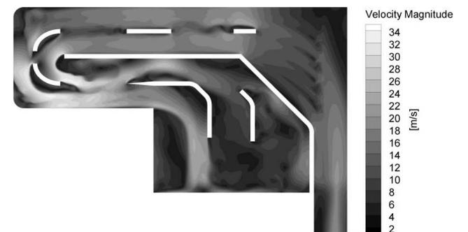
**Figure 19 – Velocity magnitude of water inside the probe in case Sim2 on design #3.**
