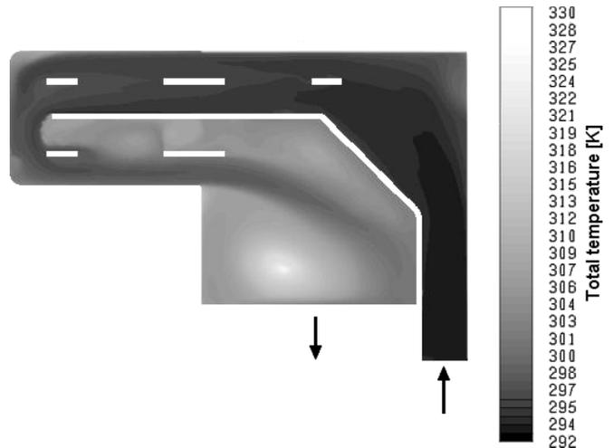
Figure 11 – Total temperature of water inside probe in case Sim2.
