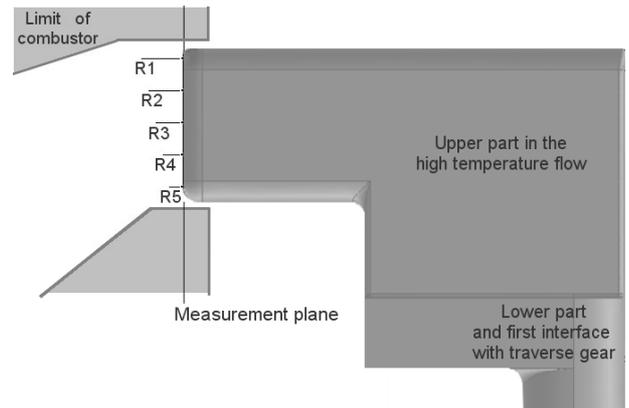
Figure 5 – External design of upper part considering the interference with the combustor, the position of the measurement plane and the radial position of the five gas sampling inlet.
