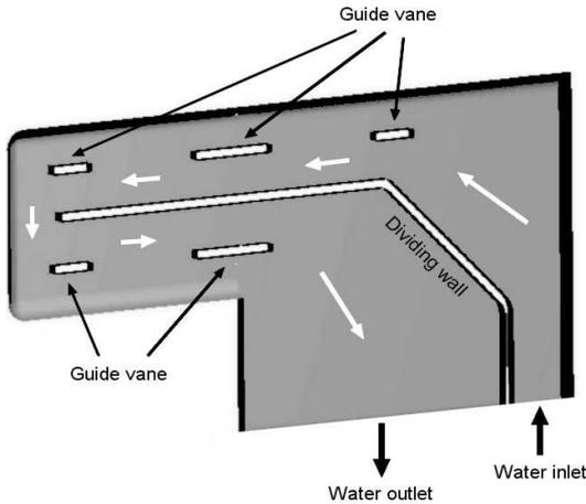
Figure 9 – Simulated volume inside the gas analysis probe with the water path.
