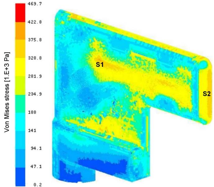
Figure 14 – Von Mises stress on the probe due to thermal expansion and internal water pressure.
