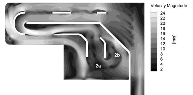
**Figure 18 – Velocity magnitude of water inside the probe in case Sim2 on design #2.**
