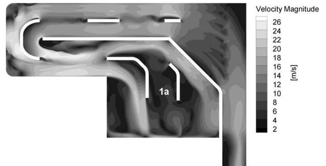
**Figure 17 – Velocity magnitude of water inside the probe in case Sim2 on design #1.**
