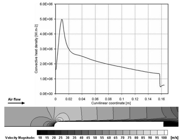
**Figure 8 – Contours of velocity magnitude around the probe and convective heat flux at design point.**
