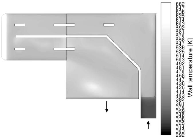
Figure 13 – External wall temperature of probe in case Sim2.
