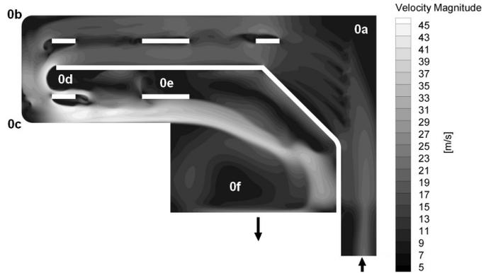
Figure 10 – Velocity magnitude of water inside probe in case Sim2.
