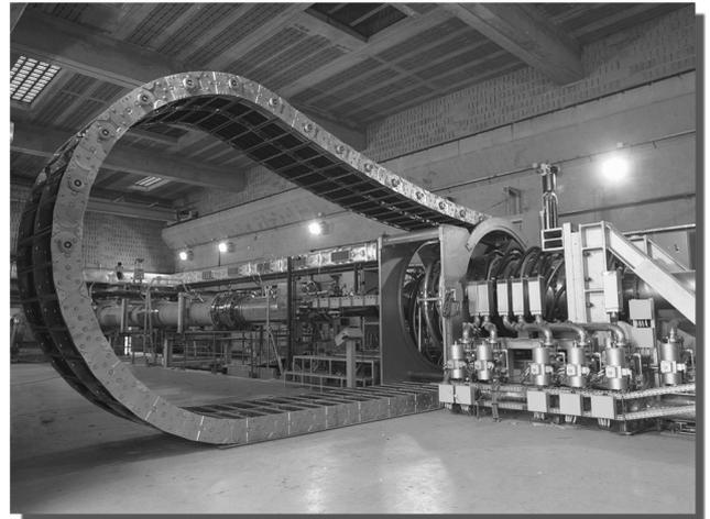
Figure 1 – K11 combustion test rig (max. inlet test conditions: 100 kg/s, 60 bars, 1073 K, max. outlet temperature: 2573 K).
