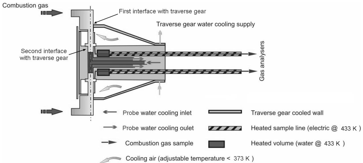
Figure 4 – Internal scheme of the K11 traverse gear with all its ancillaries.
