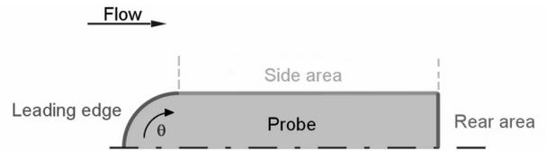
**Figure 7 – 2D geometry of the probe for computing the convective heat flux.**
