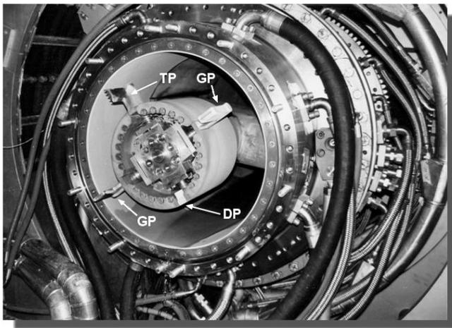
Figure 3 – Traverse gear of K11 equipped with a temperature probe (TP), 2 gas analysis probes (GP) and a dummy probe (DP).
