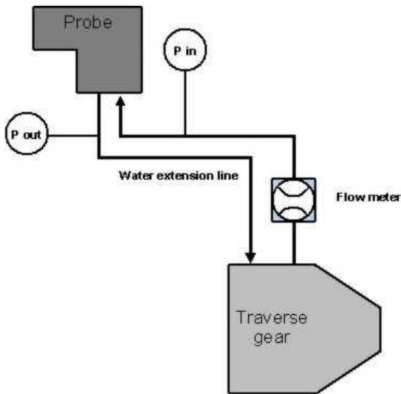
Figure 23 – Scheme of the experimental setup used for preliminary functional tests on the gas analysis probes.
