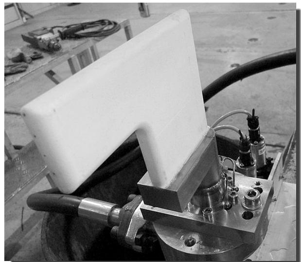
Figure 22 – NEWAC gas analysis probe during functional tests of the water cooling system. White part of the probe is a thermal barrier coating added after this study for specific test purpose.
