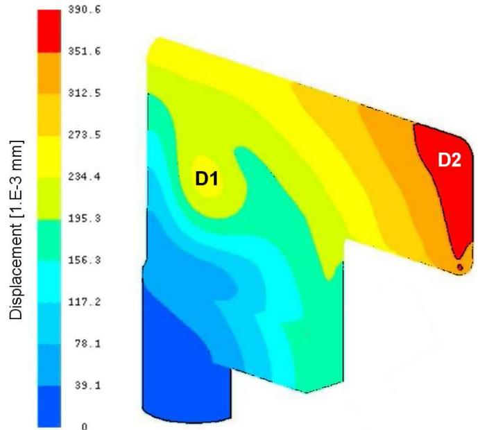
Figure 15 – Maximal displacement of the probe at design point.
