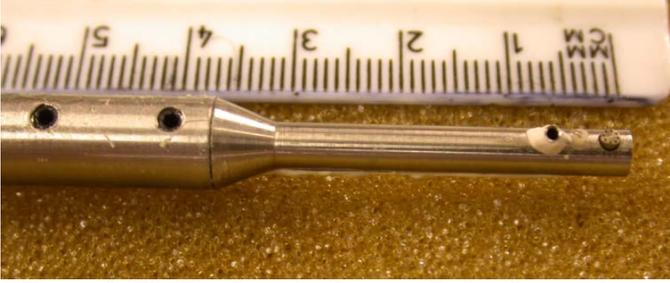
**Figure 2:** The Fast-Insertion Pressure Probe. Sensors from right to left are the Kulite XCE-77-062-10BARA high frequency transducer, the 125  $\mu\text{m}$  K-type thermocouple and the Pitot tube.
