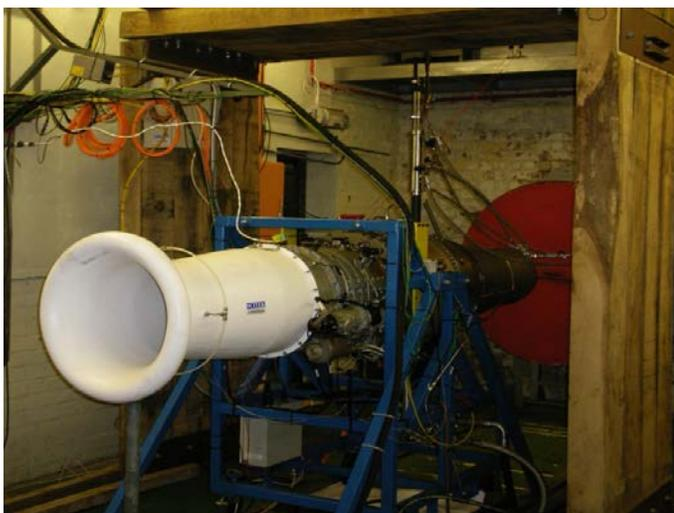
**Figure 6:** The Rolls-Royce Viper Mk201C turbojet with the traverse installed in the vertical position.
