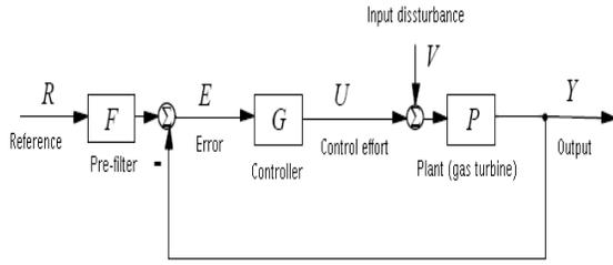
Figure5. General structure of QFT controller with uncertain plant.
