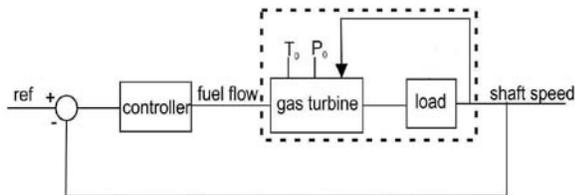
Figure1. Block diagram of the gas turbine system.
