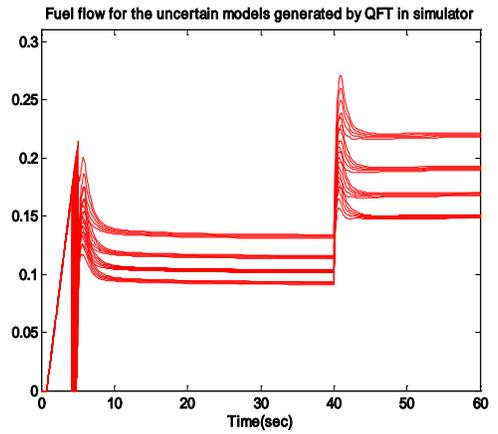
Figure10. Control effort of uncertain models generated by QFT controller in 80%NH in new simulator.
