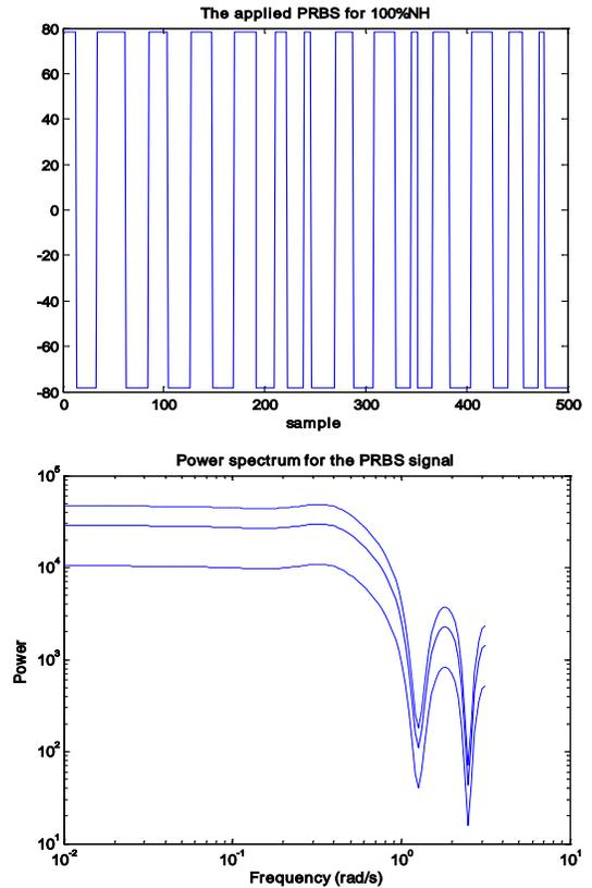
Figure3. The applied PRBS signal and its frequency spectral.
