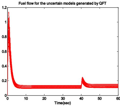
Figure7. Control effort signals for uncertain models generated by QFT controller in 80%NH.
