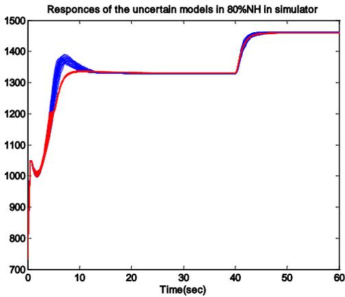
Figure9. Step responses of the uncertain models in steady state with original and new simulators.
