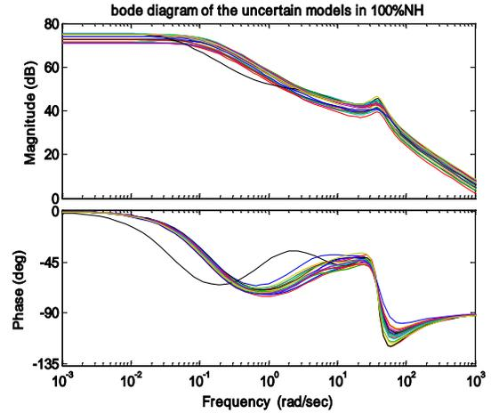
Figure4. Bode diagram of 20 sample models of uncertain gas turbine in 100%NH.
