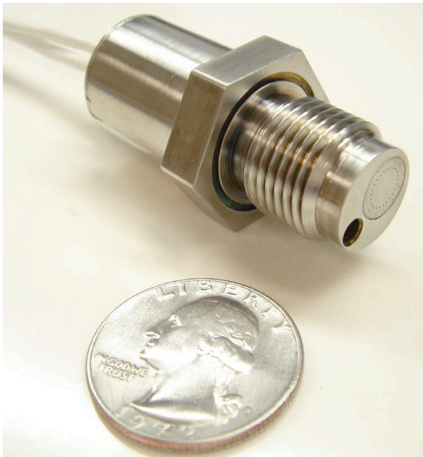
Figure 7: Photograph of fully assembled static-dynamic transducer (screen over removable filter module not shown).
