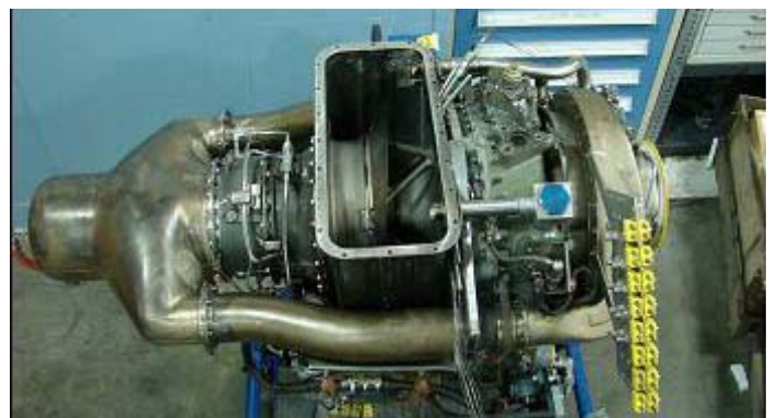
Figure 20. Test engine instrumented prior to installation in the test stand.
