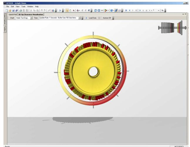
**Figure 8: example single stage view of the advanced tip clearance 3D visualization. Coloring and exaggeration can be observed.**
