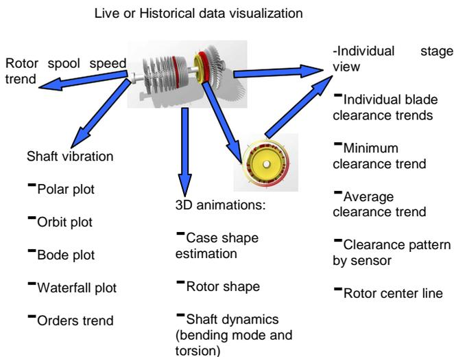
**Figure 4: the 3D visualization as a common platform to access the engine measurement and for high level animations**
