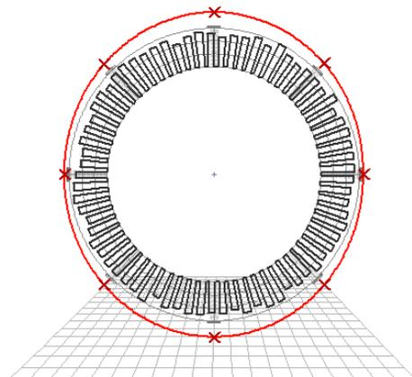
**Figure 6: overlay of an example elliptic case shape estimation on the rotor blade signature. Casing shape interpolated based on the measurement of eight sensors.**
