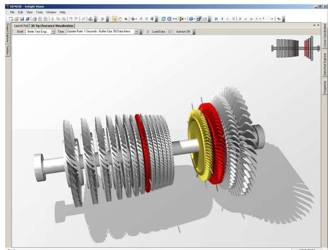
**Figure 7: example machine shaft view of the advanced tip clearance 3D visualization. The stages instrumented with tip clearance sensors are in colors.**
