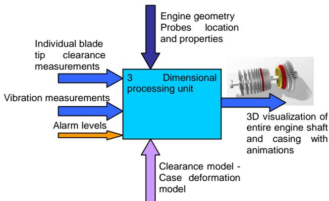
**Figure 3: black box representation of the advanced 3D visualization of the tip clearance measurements**
