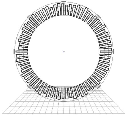
**Figure 5: representation of a stage with an example random blade pattern measured from 8 tip clearance sensors mounted each 45 degrees around the casing.**
