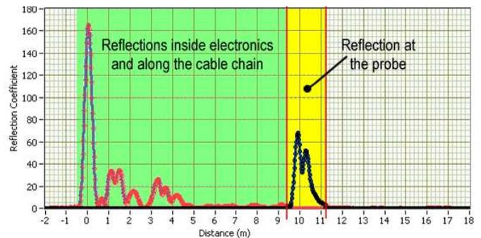
**Figure 2: Decomposition of individual reflections occurring along the cable line used for diagnostics of the microwave system.**
