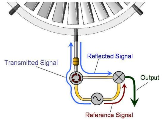
**Figure 1: Sketch of the microwave subsystem of the tip clearance measurement system.**
