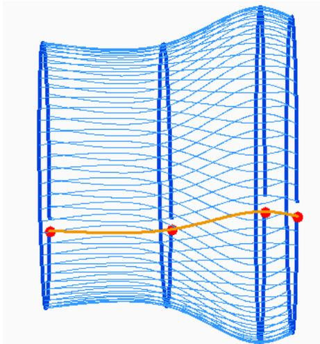
**Figure 9: Concept of 3D representation of shaft vibration orbit plots with interpolation in-between measurement plans.**
