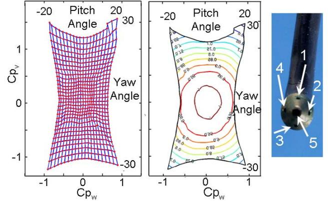
**Fig. 1: Five-hole probe hole orientation (right), flow angle -  $cp_w, cp_v$  relation (left)  $cp_5 - cp_w, cp_v$  relation (middle).**
