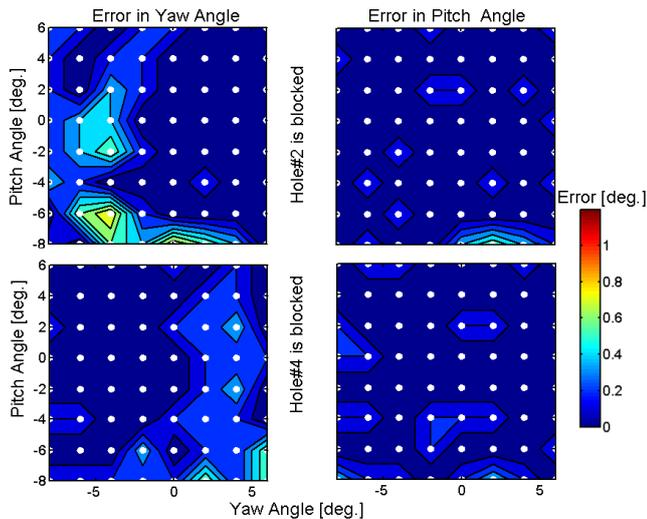
**Fig. 11: Error in yaw and pitch angle when hole number 2 and 4 is blocked**
