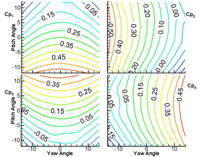
Fig. 3: Variation of non-dimensional parameters ( $cp_1$ ,  $cp_2$ ,  $cp_3$ ,  $cp_4$ ) with flow angle
