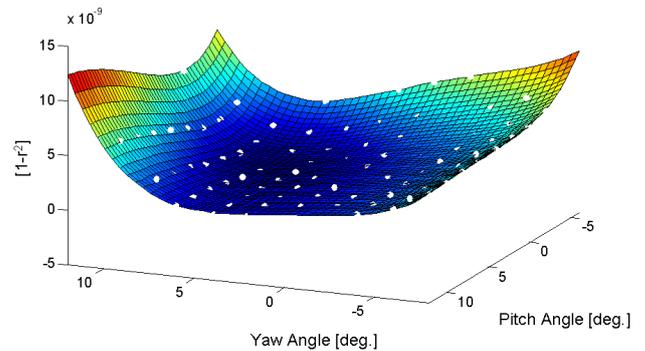
**Fig. 10: Surface fit for flow angle of 6 deg., 0 deg. with four-hole arrangement**
