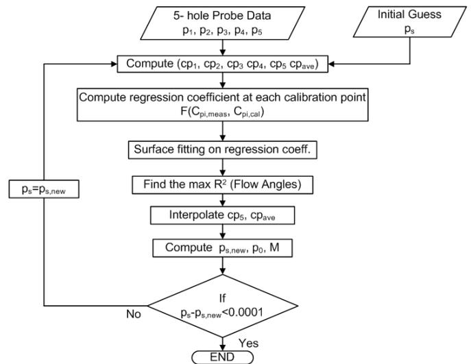
Fig. 6: New data processing algorithm
