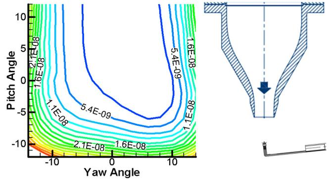
**Fig. 9: Distribution of  $(1-r^2)$  for flow angle of 6 deg., 0 deg. with four-hole arrangement**
