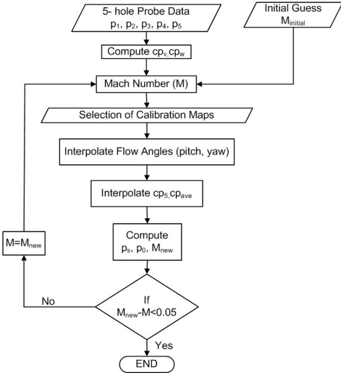
Fig. 2: Traditional data processing algorithm.
