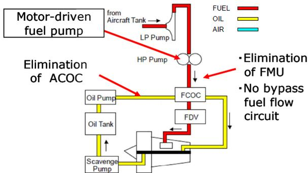
Figure 3 A highly efficient electrical fuel pump system
