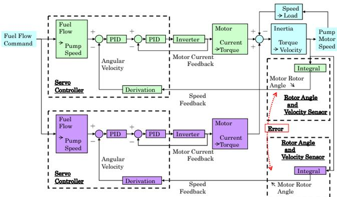
Figure 11 Simulation block diagram for the electrical motor-driven fuel pump
