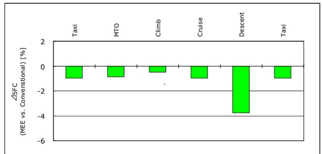
Figure 5 SFC reduction accomplished by the MEE STEP 1
