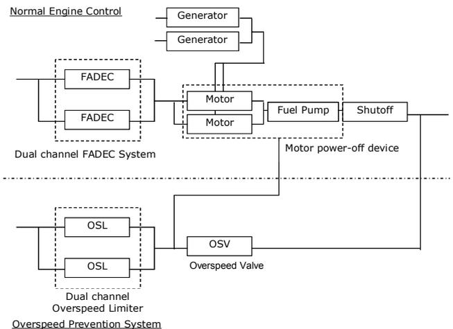
Figure 9 The MEE engine control and OSL system
