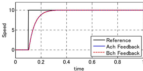
(a) Step response without feedback error between channels
