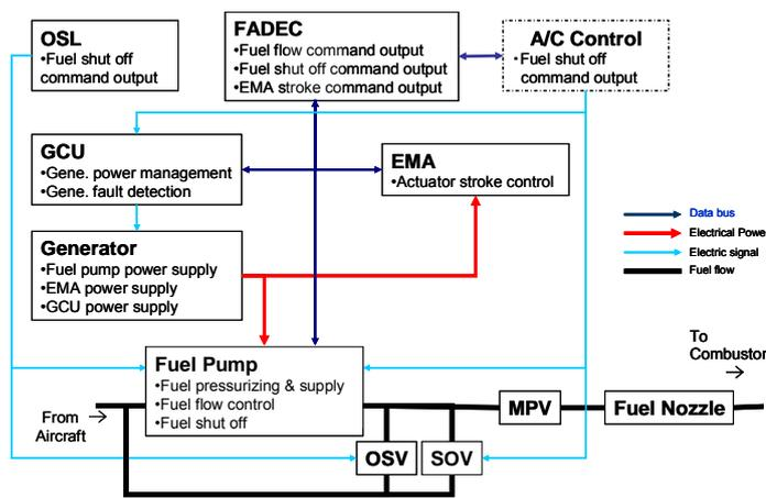
Figure 10 Typical MEE STEP 1 configuration
