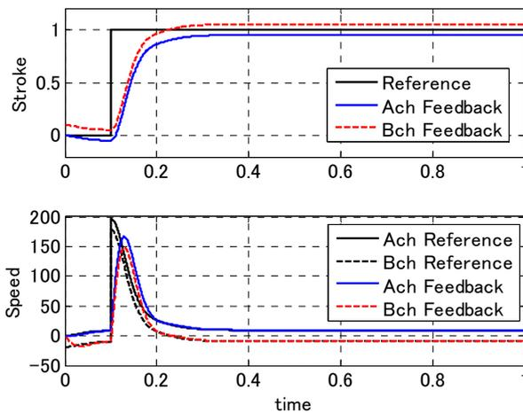
(b) Step response with feedback error between channels
