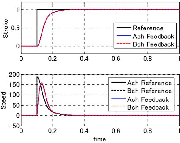
(a) Step response without feedback error between channels
