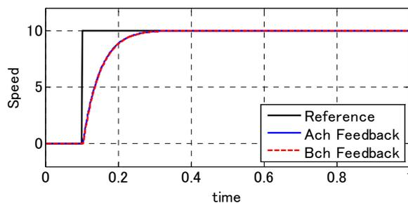
(b) Step response with feedback error between channels
