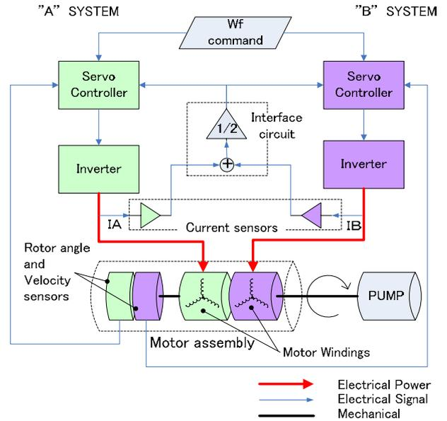
Figure 6 Block diagram of the redundant motor system
