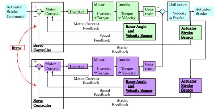
Figure 13 Simulation block diagram for the EMA
