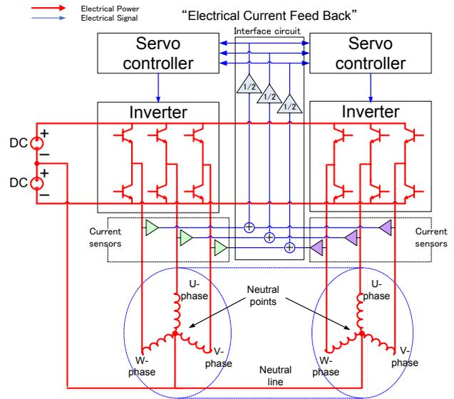
Figure 7 Active-Active control for three phase/dual motor
