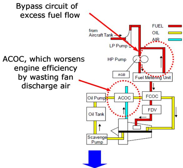
**The proposed MEE STEP 1 Electrical motor-driven fuel pump system**
