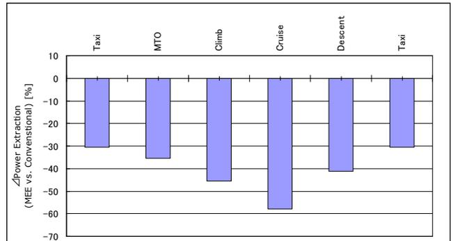
Figure 4 Reduction of power extraction from the engine
