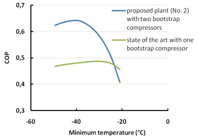
Fig. 15 – Performance comparison between the second layout and a state-of-the-art inverse Joule-Brayton plant.
