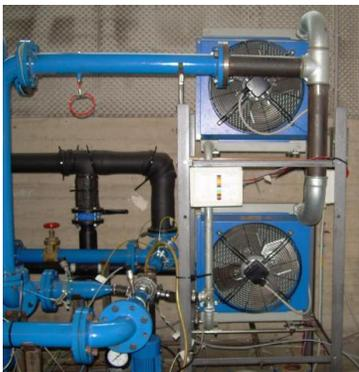
Fig. 5 – Test bench: turbocharger and fan coolers.
