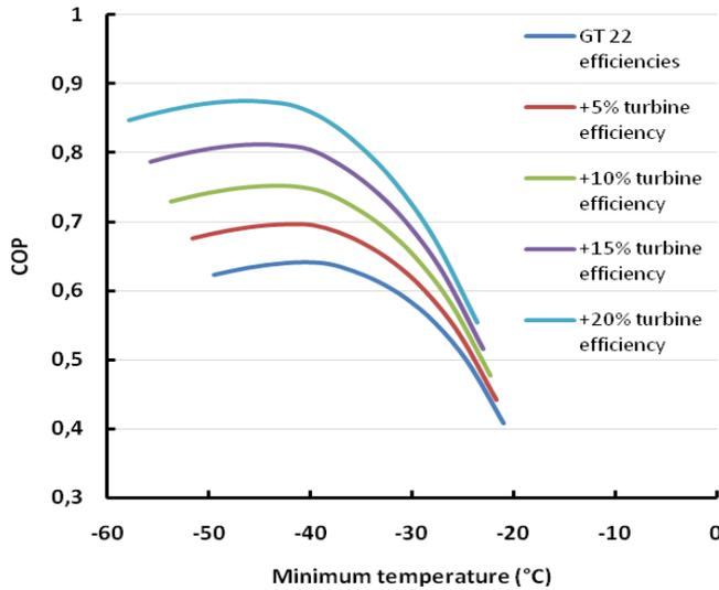
Fig. 17 – Performance of the second layout for higher values of turbine efficiency.
