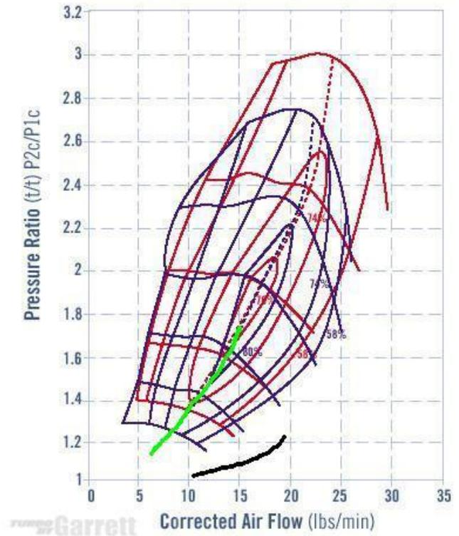
Fig. 8 – Centrifugal compressor map, courtesy Garret.
