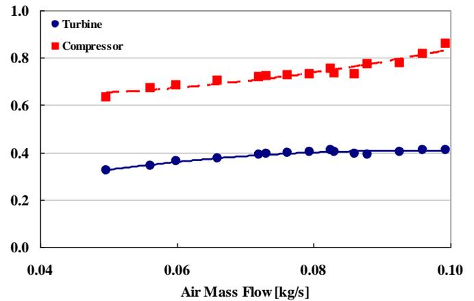
Fig. 6 – Compressor and turbine polytropic efficiencies.
