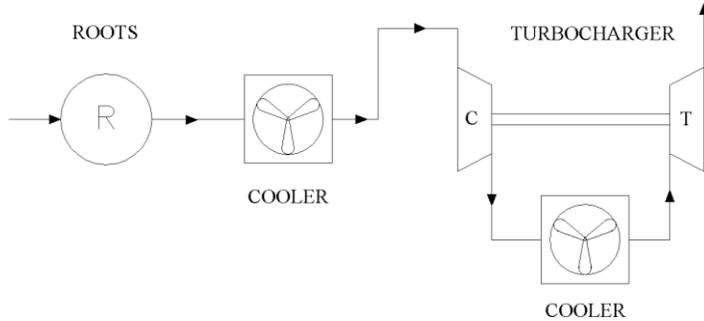
Fig. 4 – Test bench layout.
