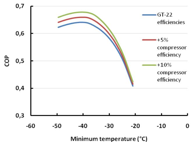
Fig. 16 – Performance of the second layout for higher values of centrifugal compressor efficiency.
