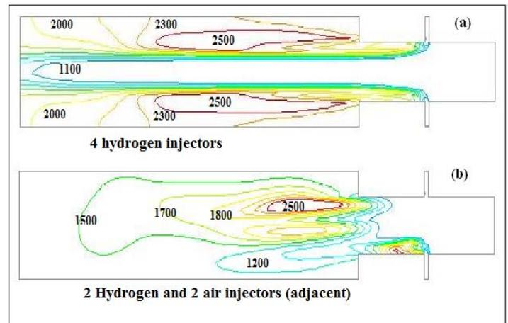
**Figure 7:** Temperature distribution along x-x axis (a) for four hydrogen injection holes (b) for two hydrogen and two air injection holes.
