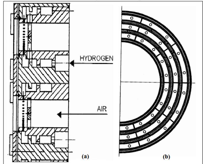
**Figure 3:** Ring-shaped structure of the micromix hydrogen combustor (Air and hydrogen admission for diffusive combustion in the micromix hydrogen combustor of third generation for the APU GTCP 36-300 engine [8]).
