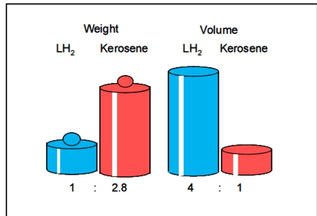
**Figure 1:** The weight and volume of kerosene and liquid hydrogen, respectively, containing the same energy content. (Illustration idea from Heinz-Günter Klug, retired from Airbus Germany.)
