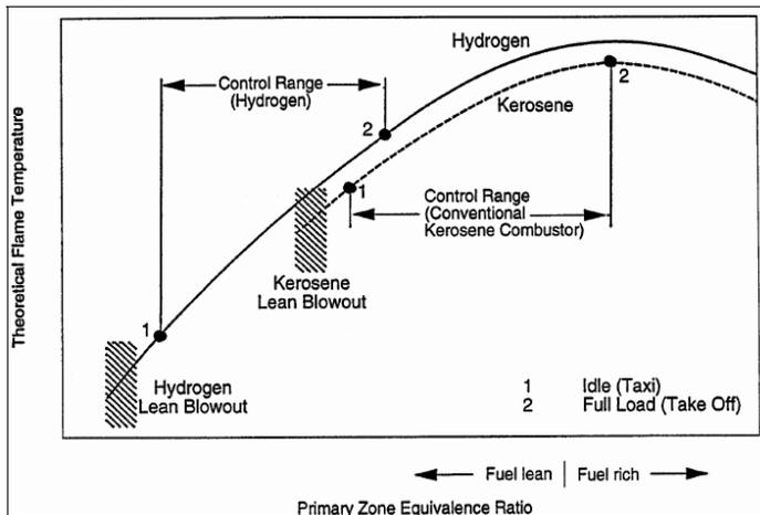
**Figure 2:** Temperature characteristics of the combustion chamber primary zone [5].
