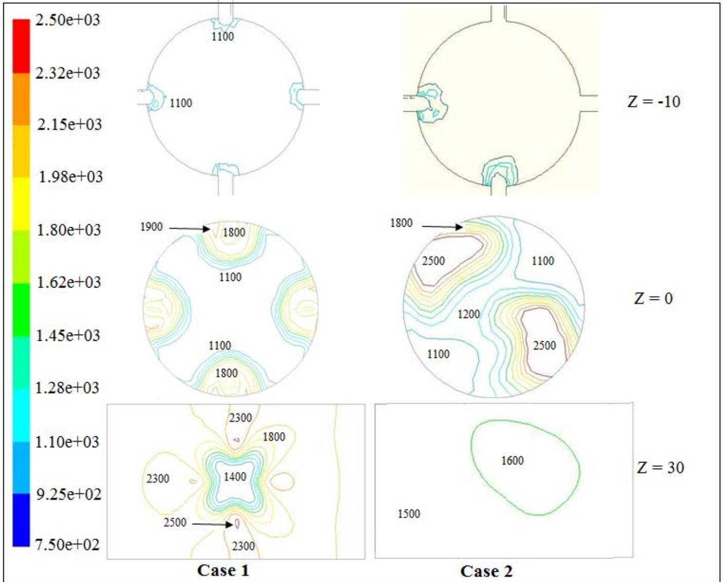
**Figure 8:** Temperature distribution at different cross sections along the  $z$  axis (a) for four hydrogen injection holes (b) for two hydrogen and two air injection holes.
