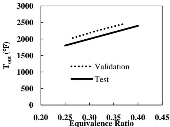
**Figure 6:** Comparison of the outlet temperature against the equivalence ratio between the validation data and the test data.
