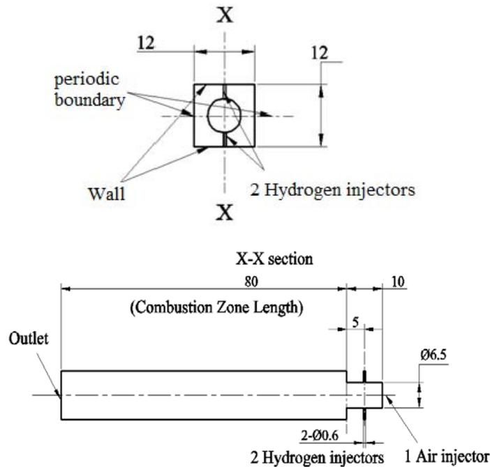
**Figure 5:** Domain geometries for the validation (mm)
