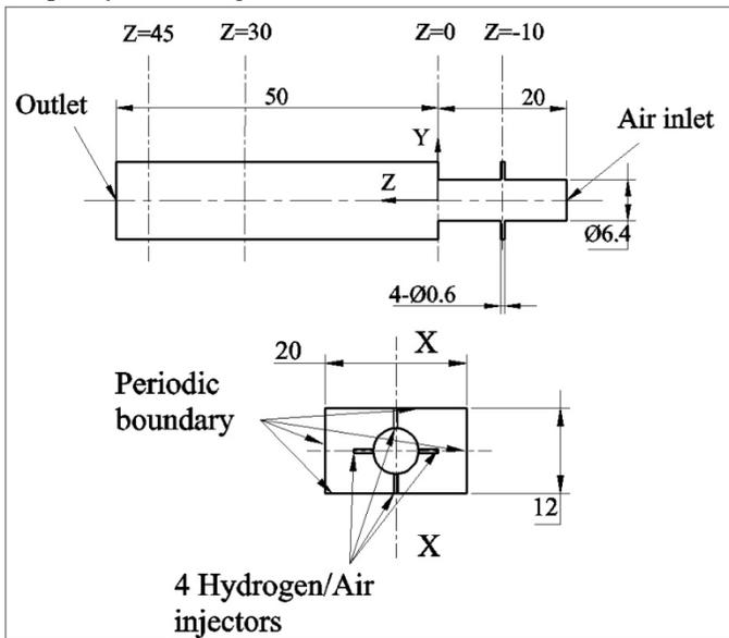
**Figure 4:** Schematic diagram of micromix combustor with rectangular prism combustion zone.
