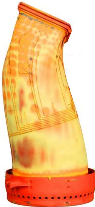
Figure 8. 9F transition piece with thermal paint
