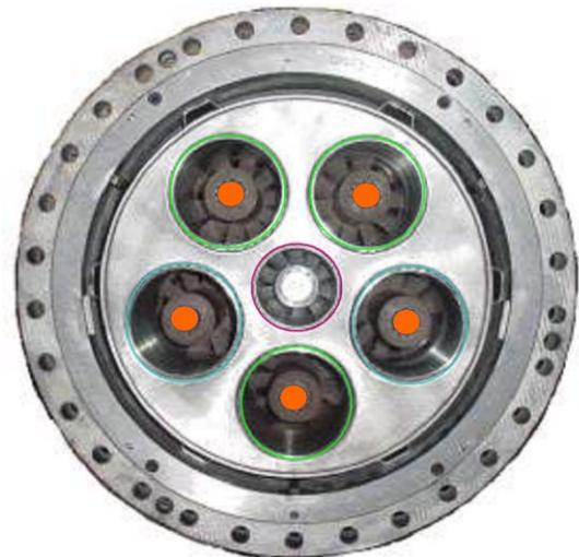
**Figure 4. DLN2.6+ Head End Arrangement**
