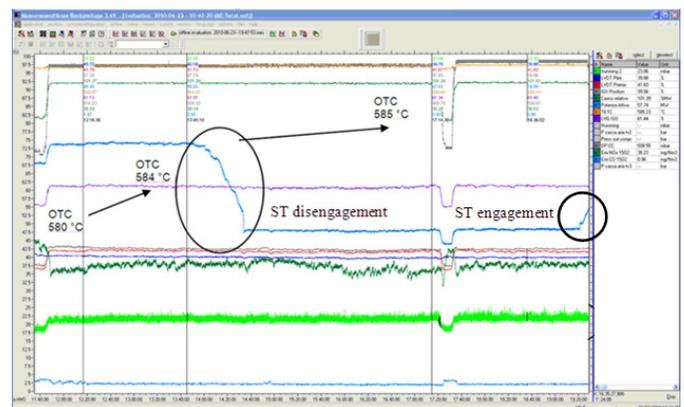
Figure #13. Maximum turbine outlet temperature optimization at the base load
