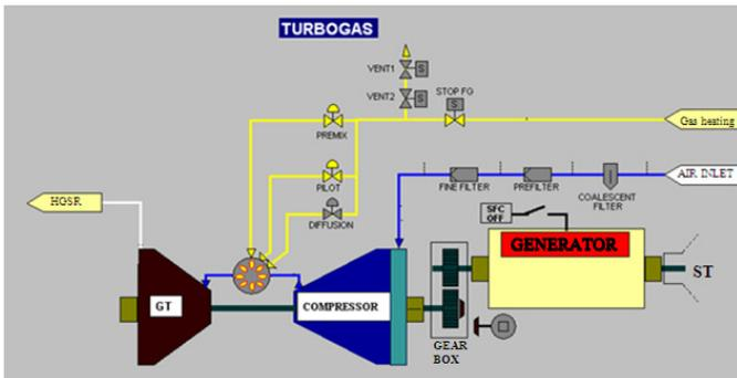
Figure #2. Gas turbine power block
