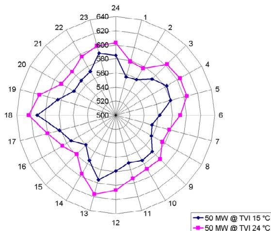
Figure #11. Turbine outlet temperature dependence with the ambient temperature at 50 MW
