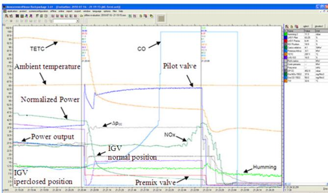
Figure #15. Load rejection test
