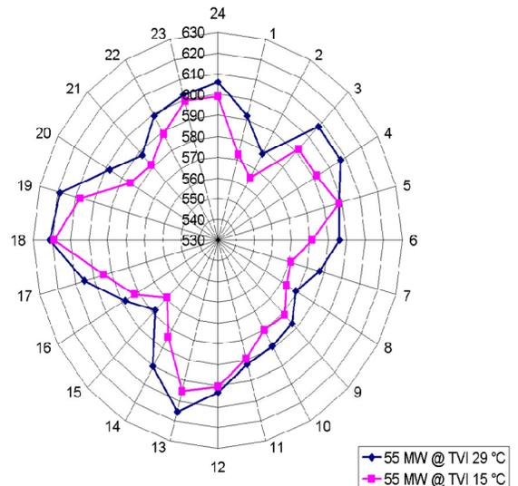
Figure #12. Turbine outlet temperature dependence with the ambient temperature at 55 MW
