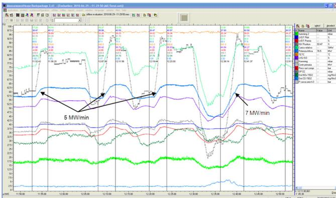
Figure #14. Ramping of the gas turbine during commercial operation
