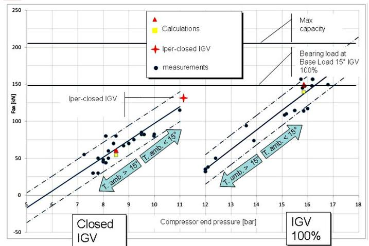
Figure #5. Axial bearing load
