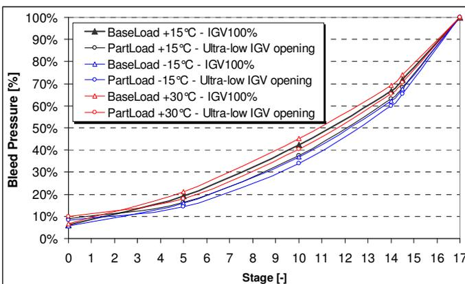
Figure #4. Bleed pressure levels at extraction points
