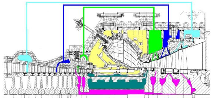
Figure #3. Flow path of cooling/sealing air in the AE64.3A GT
