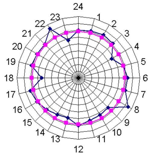
Figure #8. Turbine outlet temperature distribution at FSNL
