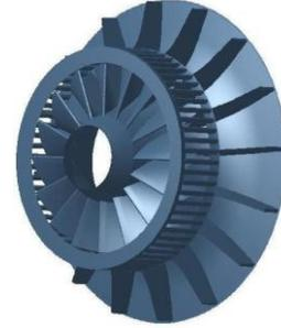
Fig. 3 Compressor with holed casing treatment
