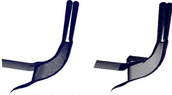
Fig. 4 Grids of single impeller passage
