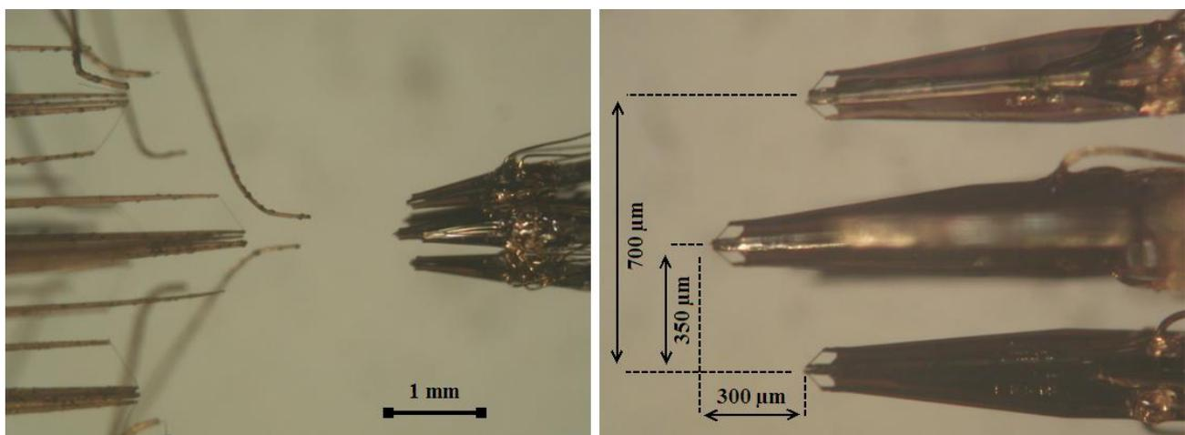
**Figure 1.** Micro-photo of a micro-machined probe next to a conventional one (left). Array separation dimensions of the micro-machined probe (right).
