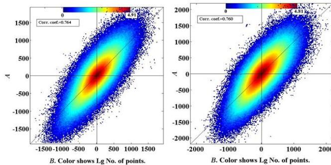
**Figure 2.** Examples of joint PDFs of  $A = \partial u_1 / \partial x_1$  and  $B = -(\partial u_2 / \partial x_2 + \partial u_3 / \partial x_3)$ . Wind tunnel experiments. Left – at 20 mm from rough wall, right – at 7.5 mm from smooth wall.
