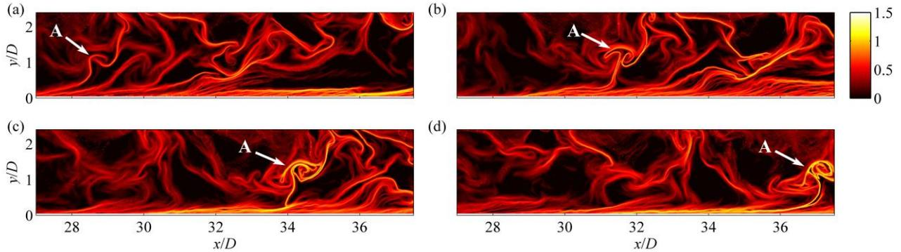
**Figure 3.** A single hairpin vortex in the transitional boundary layer. Arrow A indicates the head of the hairpin vortex. The integration time length is  $T = -4.0$ s (backward integration).
