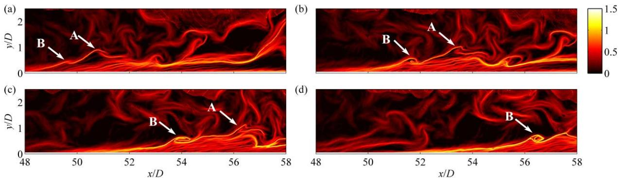
**Figure 4.** Hairpin vortex packet in the turbulent boundary layer. Arrows A and B indicate two successive hairpin heads in the packet. The integration time length is  $T = -4.0$ s (backward integration).
