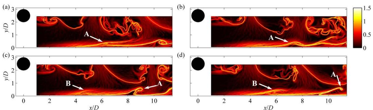
Figure 2. Lagrangian coherent structures revealed by FTLE in the boundary layer downstream of the cylinder. Arrows A and B indicate the secondary vortices induced by the wake vortices. The integration time length is  $T=-4.0\text{s}$  (backward integration).
