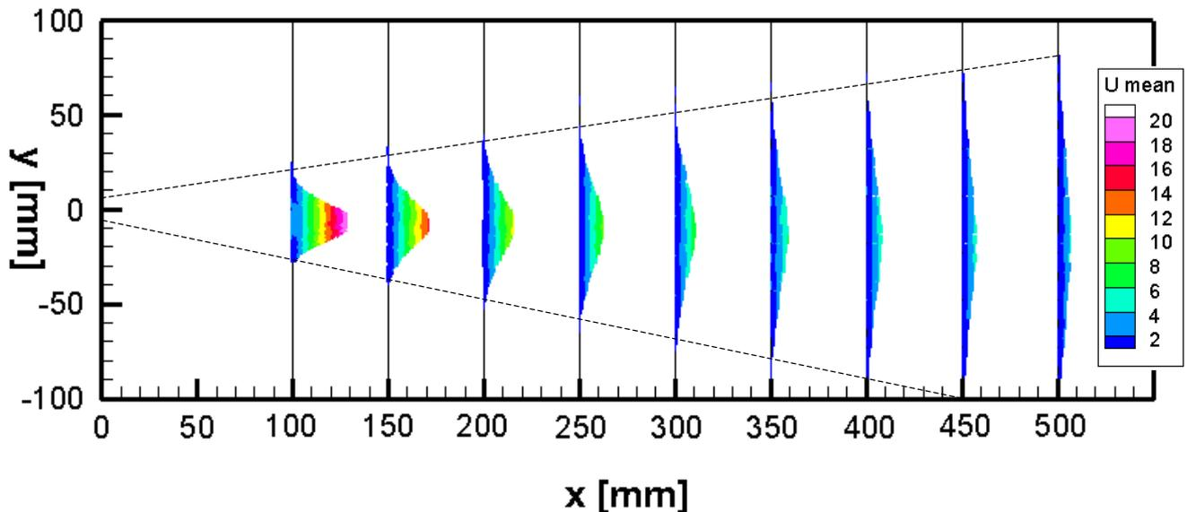
**Figure 1.** Evolution of the jet profile in the streamwise direction. The nozzle is located at  $x,y=0$ .
