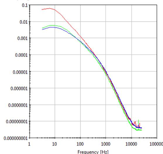
**Figure 2.** PSD for each velocity component ( $u$ -,  $v$ -,  $w$ -), at  $x=300$ mm and  $42$ mm from the jet axis.
