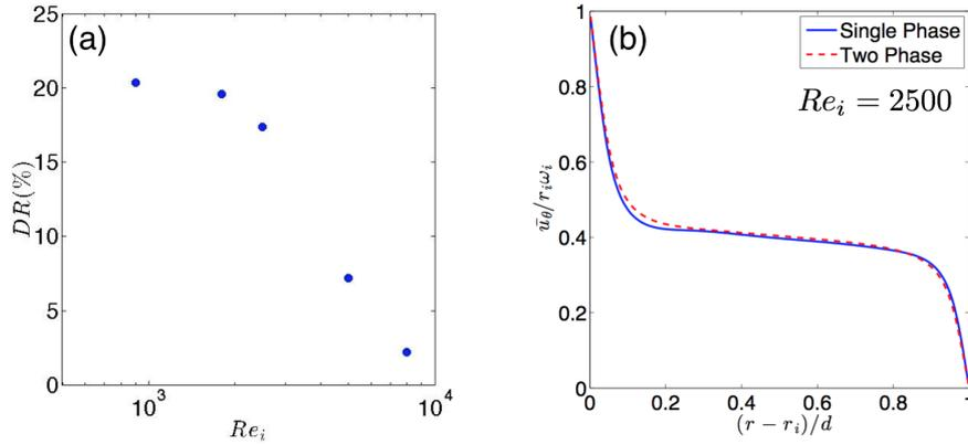
**Figure 1.** (a) Drag reduction (DR) versus the inner cylinder Reynolds number ( $Re_i$ ) (b) Normalized average azimuthal velocity versus the radial position at  $Re_i = 2500$  for both single phase and two-phase cases
