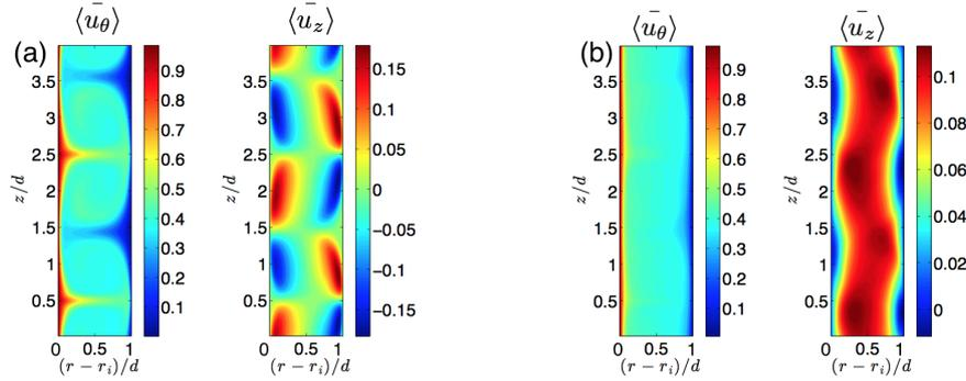
**Figure 2.** Contour fields of averaged azimuthal and axial velocity fields in the  $r$ - $z$  plane at  $Re_i = 2500$  (a) Single phase (b) Two phase.
