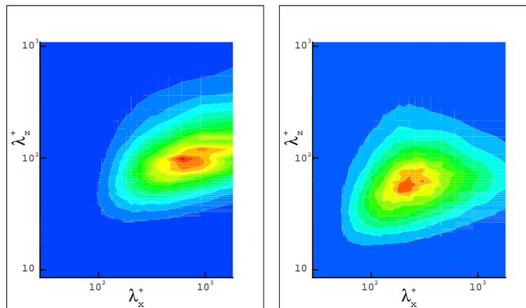
**Figure 2.** Premultiplied 2-dimensional power spectra of turbulent fluctuations (left) and perturbation field at linear stage of evolution (right) at  $y^+ = 12$ .
