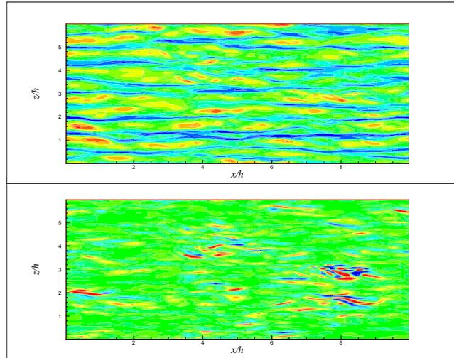
**Figure 1.** Instantaneous  $u_x$ -velocity distribution at  $y^+ = 12$  in turbulent flow (up) and in perturbation field at linear stage of evolution (down).
