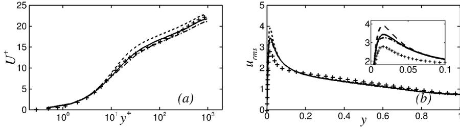
**Figure 1.** Channel flow,  $Re_\tau = 1,000$ ,  $64 \times 97 \times 64$  grid points. Mean velocity (a) and  $u_{rms}$  velocity (b). — Local ILSA with  $s_\tau^\Omega = 0.022$ ; - - - global ILSA model [4] with  $s_\tau^V = 0.022$ ; - - - dynamic model [1]; + DNS [2].
