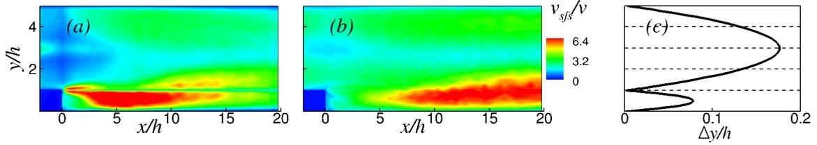
**Figure 2.** Ratio of the eddy viscosity ( $\nu_{sfs}$ ) to the kinematic viscosity for the backward-facing step on the coarse grid using (a) the dynamic model and (b) the local ILSA model with  $s_\tau^\Omega = 0.022$ . (c) grid size across the domain ( $1.3 \times 10^{-3} \leq \Delta y/h \leq 0.18$ ).
