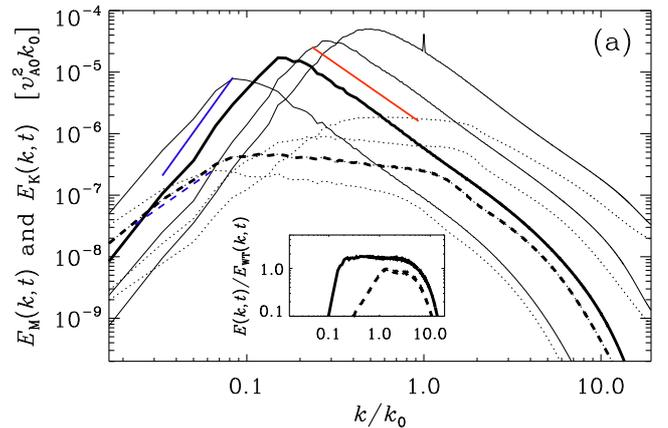
**Figure 1.** Magnetic (solid lines) and kinetic (dashed lines) energy spectra for Run A at times  $t/\tau_A = 18, 130, 450$ , and  $1800$ ; the time  $t/\tau_A = 450$  is shown as bold lines. The straight lines indicate the slopes  $k^4$  (solid, blue),  $k^2$  (dashed, blue), and  $k^{-2}$  (red, solid). The inset show  $E_M$  and  $E_K$  compensated by  $E_{\text{WT}}$ .
