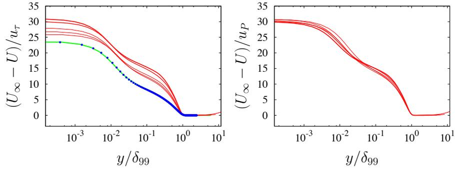
**Figure 2.** Mean velocity defect profiles in inner wall ( $u_\tau$ ) and pressure velocity ( $u_p$ ) scaling. ZPG TBL DNS of Jiménez et al. [3] - blue dots; ZPG TBL DNS current simulation - green line; APG TBL DNS from current simulation at different stream wise locations - red lines.
