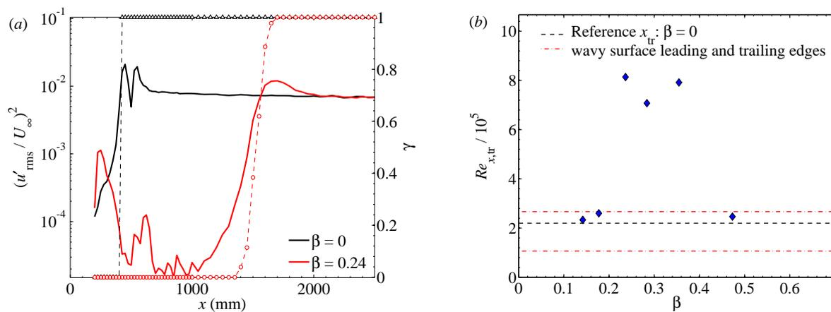
**Figure 2.** Transition measurements with  $U_\infty = 8$  m/s,  $F = 162$ . (a) Streamwise energy evolution (solid lines) and intermittency (dashed lines) plotted for the flat plate reference case ( $\Delta$ ) and for the wavy surface case ( $\circ$ ) with  $\beta = 0.24$ . (b) Transition Reynolds numbers for a set of wavy surfaces.
