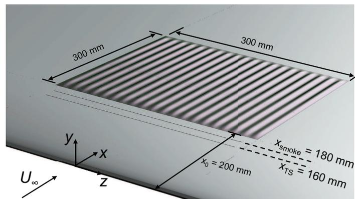
**Figure 1.** Drawing of the experimental setup showing the flat plate with wavy surface insert, and positions of the slots for smoke injection and TS-wave excitation.
