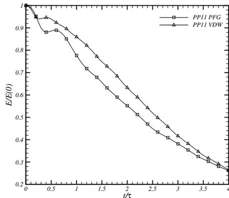
Figure 1: Turbulent kinetic energy decay.
