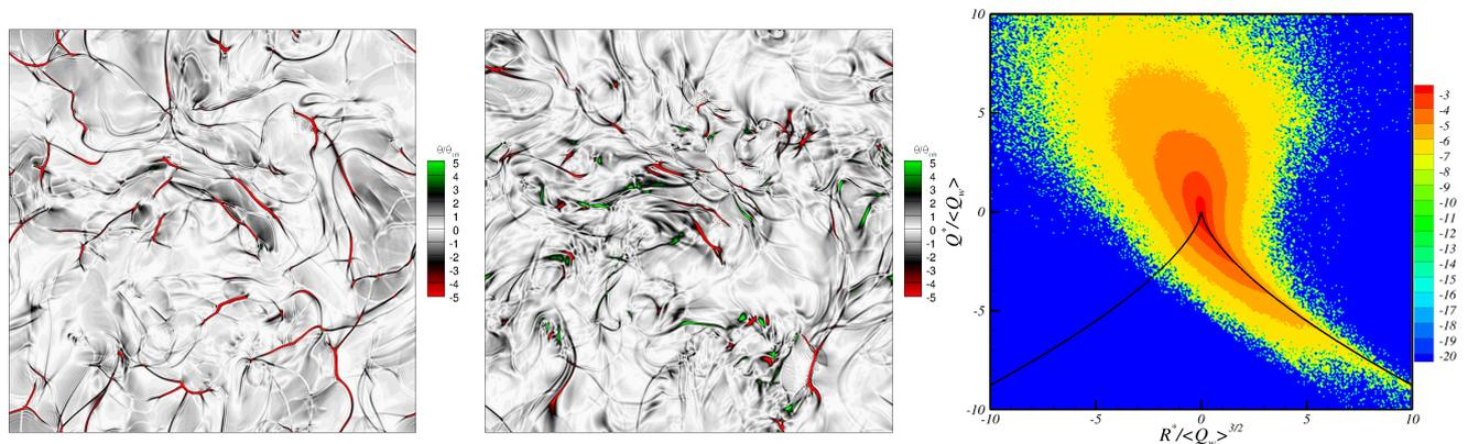
Figure 2: Ratio of dilatation to RMS dilatation for PFG EoS (left) and VDW EoS (center) for fluid PP9 at dimensionless time  $t=1$ . Right:  $\log_{10}$  PDF ( $R^*, Q^*$ ) for PP11 VDW case.
