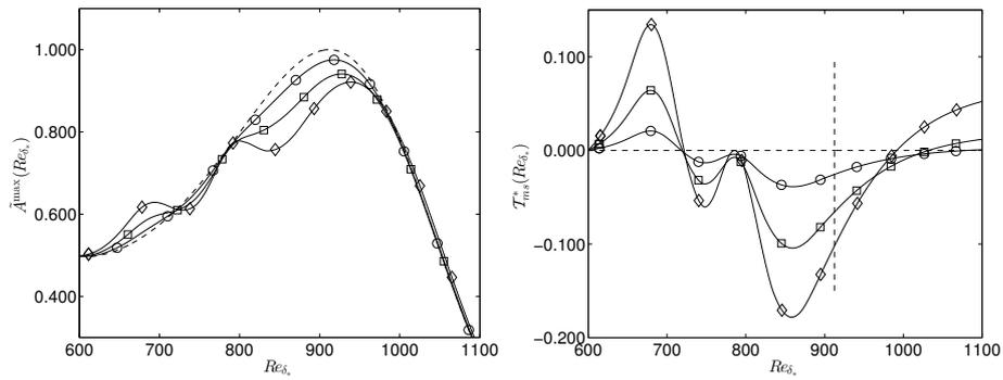
**Figure 1.** Results of linear analyses: (Left) Envelopes of Tollmien-Schlichting waves; (Right) Behaviours of transmitted Tollmien-Schlichting waves
