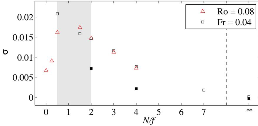
**Figure 1.** Marino et al., 2013. Growth rate of the kinetic energy as a function of  $N/f$  for a variety runs. Empty symbols correspond to  $512^3$  runs, the filled to  $1024^3$  runs. Same values of  $N/f$  are obtained for different combinations of the Froude ( $Fr$ ) and Rossby ( $Ro$ ) numbers. The gray band indicates the range  $1/2 < N/f < 2$ , where the energy grows faster.
