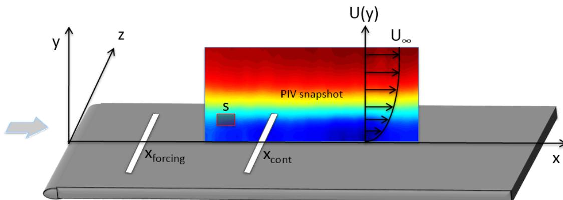
**Figure 1.** Sketch of the experimental setup and definition of the PIV window and local sensor *s*.
