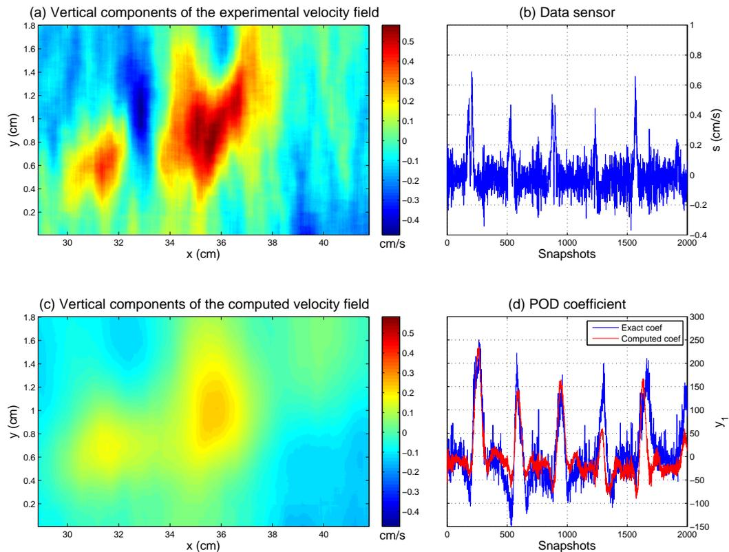
**Figure 2.** Vertical components of the experimental velocity field (a) and computed velocity field (c). Data sensor (b). Experimental and computed first POD coefficient (d).
