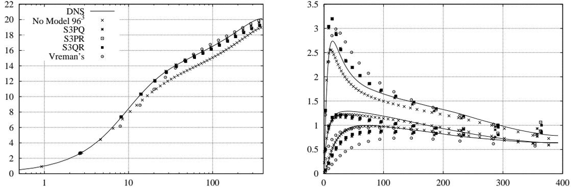
**Figure 2.** Results for a turbulent channel flow at  $Re_\tau = 395$  obtained with a  $32^3$  mesh for LES and a  $96^3$  mesh without model, i.e.  $\nu_e = 0$ . Solid line corresponds to the DNS by Moser *et al.* [2].
