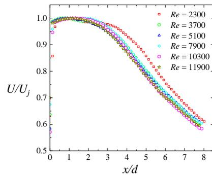
**Figure 1.** Streamwise mean velocity profile along centerline (at  $y/d = 0$ ).
