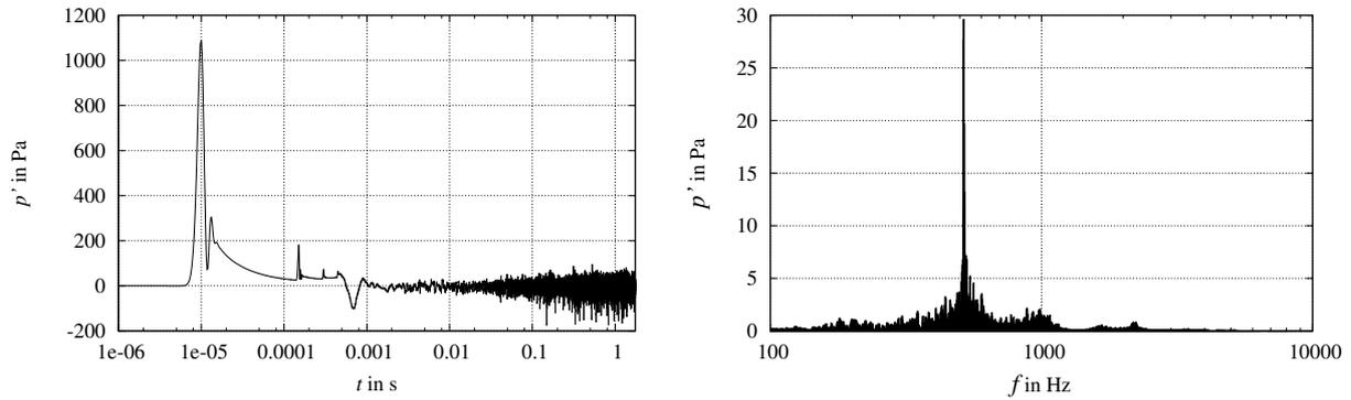
**Figure 2.** Left: Pressure fluctuations  $p'$  at point A plotted versus time  $t$ . Right: Frequency spectrum of pressure fluctuations at point B for quasi periodic state, both for  $u_0 = 15$  m/s.
