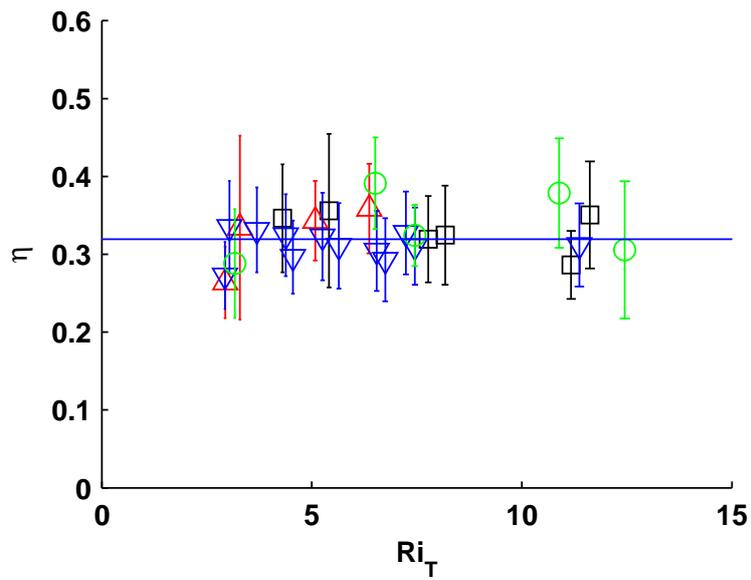
**Figure 2.** Plot of the mixing efficiency vs.  $Ri_T$ . A constant fit is also plotted as the solid back line with value 0.319.
