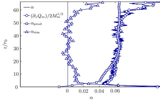
**Figure 1.** Decomposed turbulent entrainment coefficient in a steady jet at  $\text{Re} = 6815$ .
