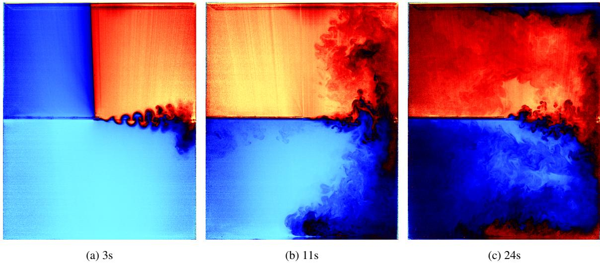
Figure 2: LIF half opening experiment at  $A = 5 \times 10^{-3}$  with rhodamine dye added to the upper layer. The colour scheme goes from turquoise for  $\rho_L(t = 0)$  through black when it is perfectly mixed to light red for  $\rho_U(t = 0)$ .
